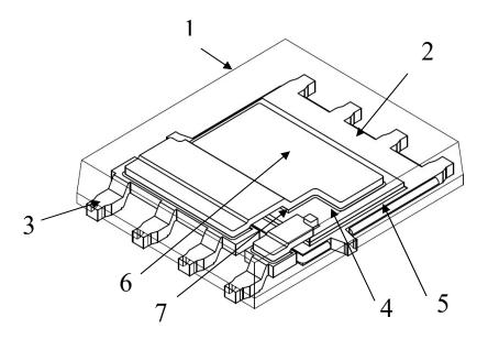
A direction of die bonding, a shape of frame and clip, die size and the number of clips differ by P/N.
