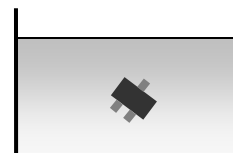
Wash off flux in 2-propanol
