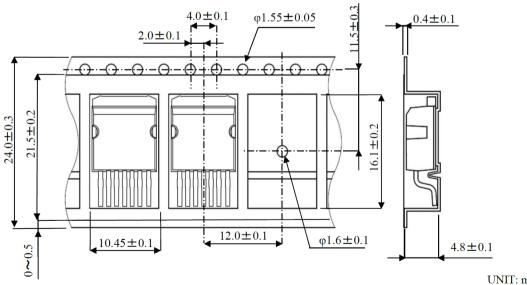
Note) Sprocket holes might be covered with the cover tape.
