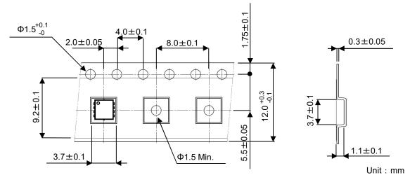
Note) Feed holes might be cover with the adhesive tape, but nothing will affect for using by that.
