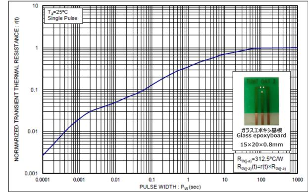
2. Transient Thermal Resistance / 過渡熱抵抗
