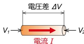
$$\text{電気抵抗 } R = \frac{V_1 - V_2}{\text{電流 } I} = \frac{\text{電圧差 } \Delta V}{\text{電流 } I} \quad [V/A]$$
