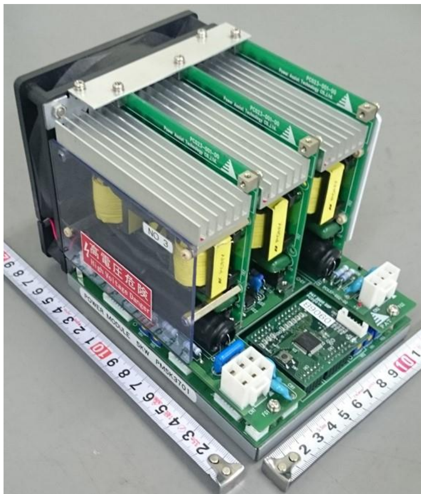
Figure 1. A view of the 5-kW LLC dc/dc using SiC MOSFETs.
