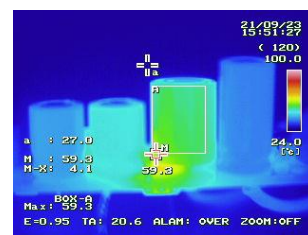
Figure 27. Each device Temperature with maximum output current
