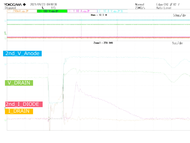
Figure 13. Vds and IL VIN = 264 Vac, IOUT = 0 A
