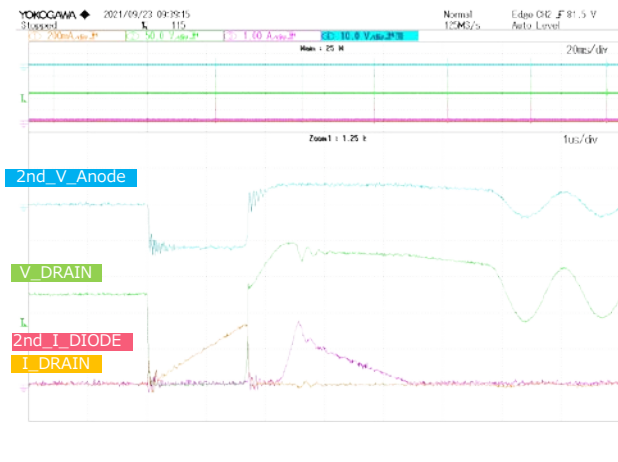
Figure 12. Vds and IL VIN = 90 Vac, IOUT = 0 A
