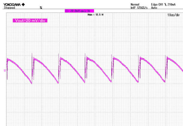
Figure 27. Vout Ripple Voltage (5MHz filter) VIN = 264 Vac, IOUT = 0.35 A
