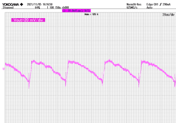
Figure 26. Vout Ripple Voltage (5MHz filter) VIN = 264 Vac, IOUT = 0.417 A
