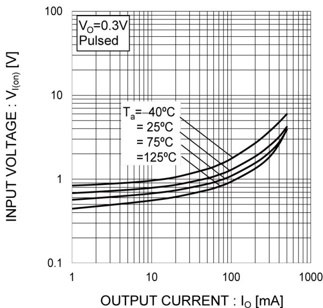
Fig.2 Output Current vs. Input Voltage
