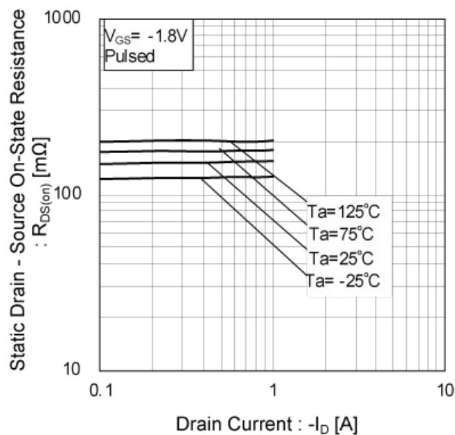
Fig.18 Static Drain - Source On - State
