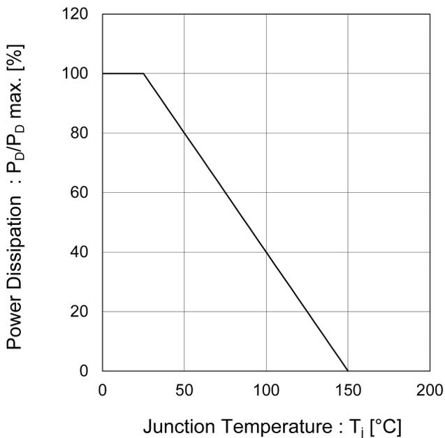
Fig.2 Drain Current Derating Curve vs. Junction Temperature
