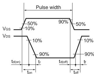
Fig.1-2 Switching Waveforms
