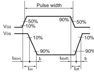
Fig.1-2 Switching Waveforms
