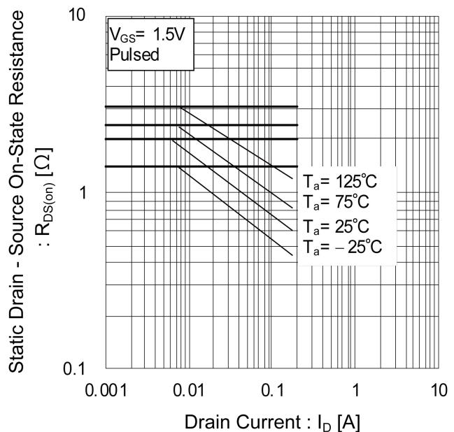
Fig.15 Static Drain - Source On - State
