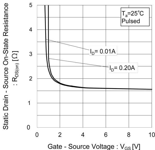
Fig.10 Static Drain - Source On - State
