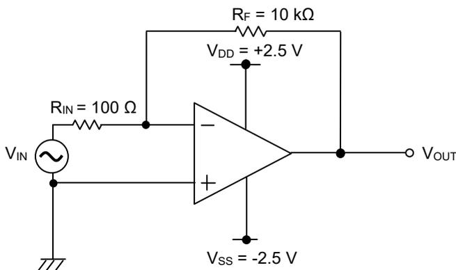
$$V_{OUT} = -\frac{R_F}{R_{IN}} V_{IN}$$
