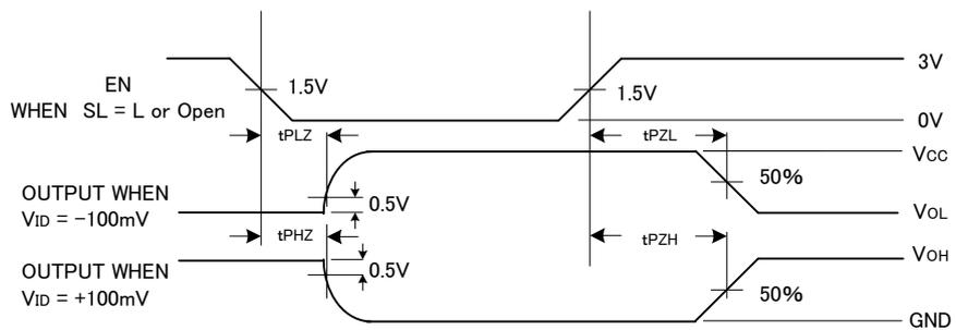
Fig.7 Receiver 3-STATE Delay Waveforms
