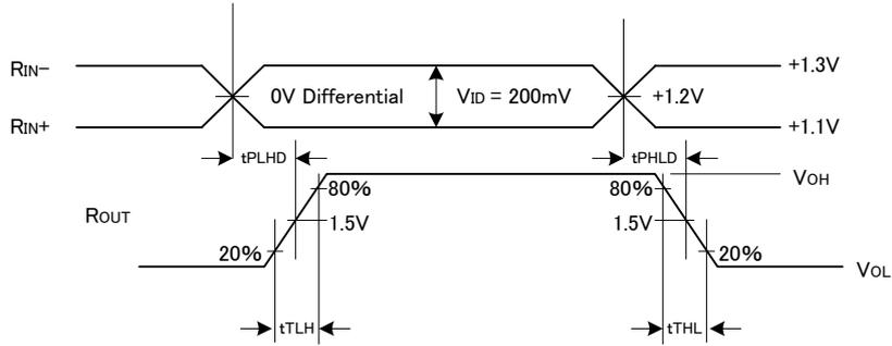
Fig.5 Receiver Propagation Delay and Transition Time Waveforms
