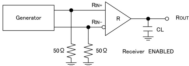
Fig.4 Receiver Propagation Delay and Transition Time Test Circuit
