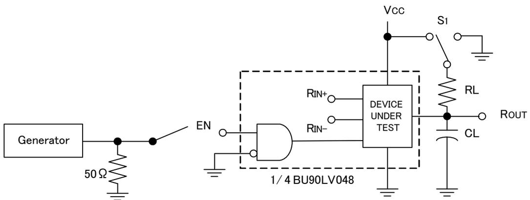
Fig.6 Receiver 3-STATE Delay Test Circuit
