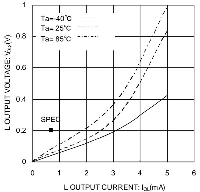
Figure 7. “L”出力電圧 2  $V_{OL2}$  ( $V_{CC}=1.6\text{V}$ )
