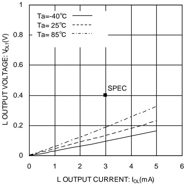
Figure 6. “L”出力電圧 1  $V_{OL1}$  ( $V_{CC}=2.5\text{V}$ )
