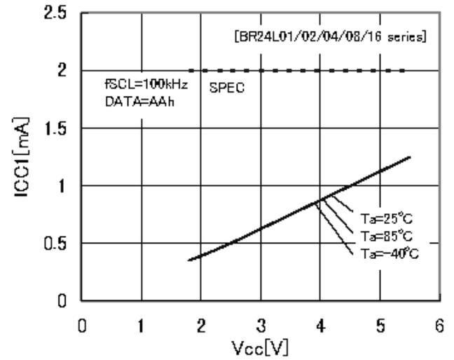
Figure 11. Current consumption at WRITE action ICC1 (fscL=100kHz)
