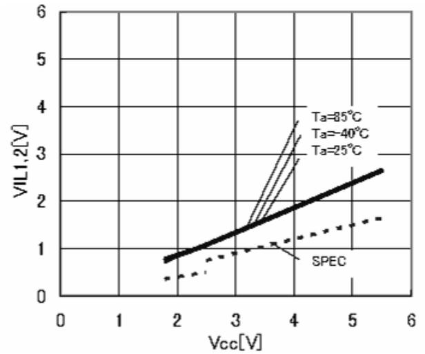
Figure 3. "L" Input Voltage  $V_{IL1,2}$
