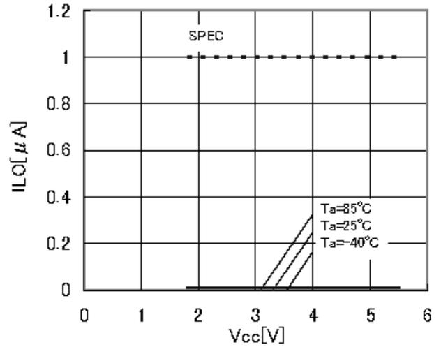
Figure 7. Output Leak Current I<sub>LO</sub> (SDA)
