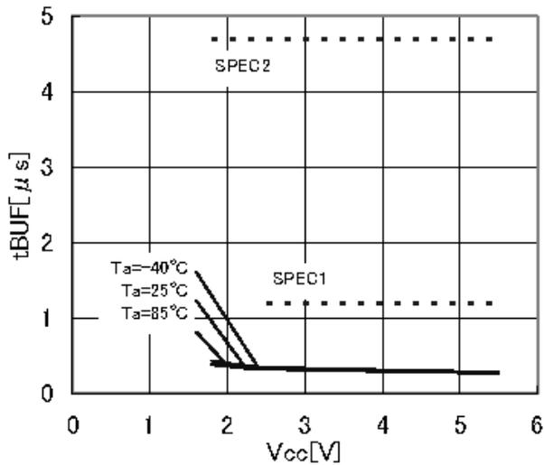
Figure 26. Bus release time before transfer start tBUF
