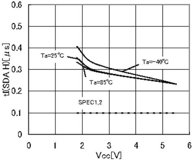
Figure 30. Noise removal valid time  $t_I(\text{SDA H})$
