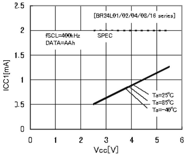
Figure 8. Current consumption at WRITE action ICC1 (f<sub>scl</sub>=400kHz)
