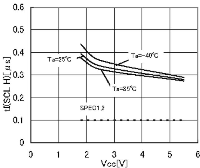
Figure 28. Noise removal valid time tI (SCL H)
