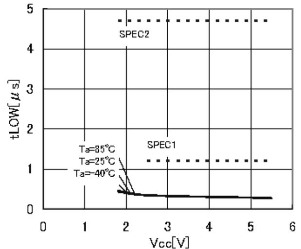
Figure 17. Data clock "L" time tLOW
