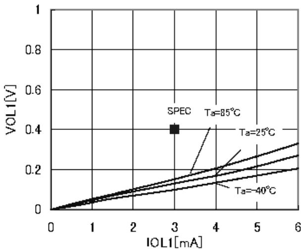
Figure 4. "L" Output Voltage1  $V_{OL1}$ - $I_{OL1}$
