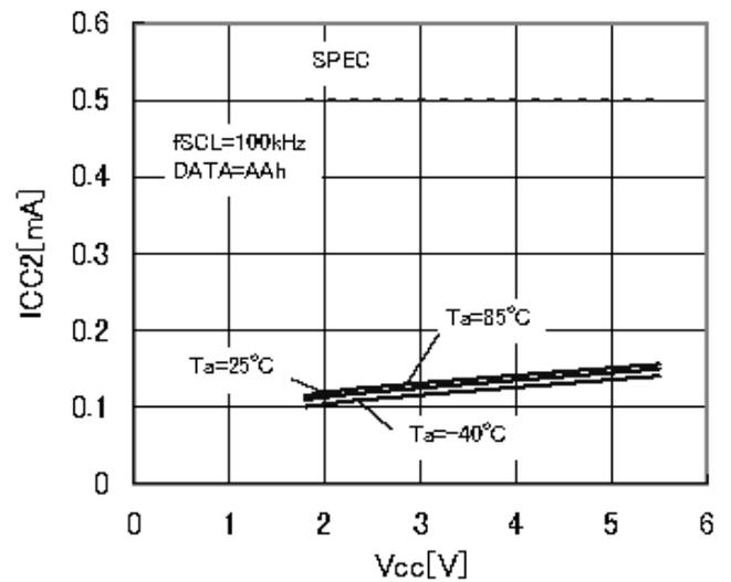
Figure 13. Current consumption at READ action ICC2 (fscL=100kHz)
