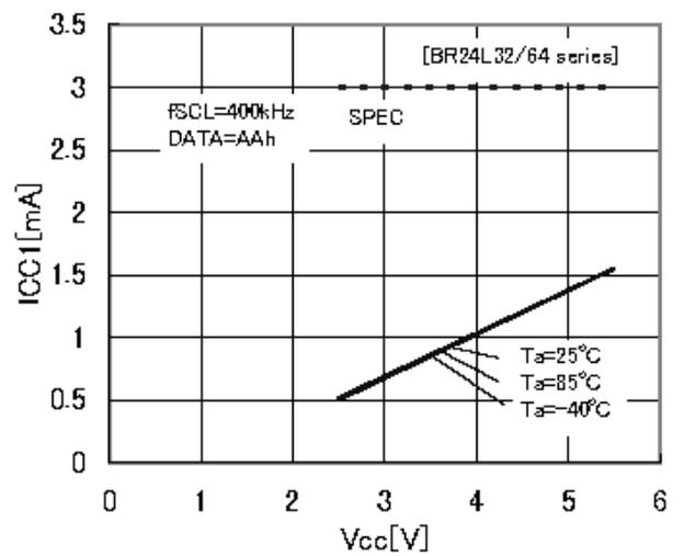
Figure 9. Current consumption at WRITE action ICC1 (f<sub>scl</sub>=400kHz)
