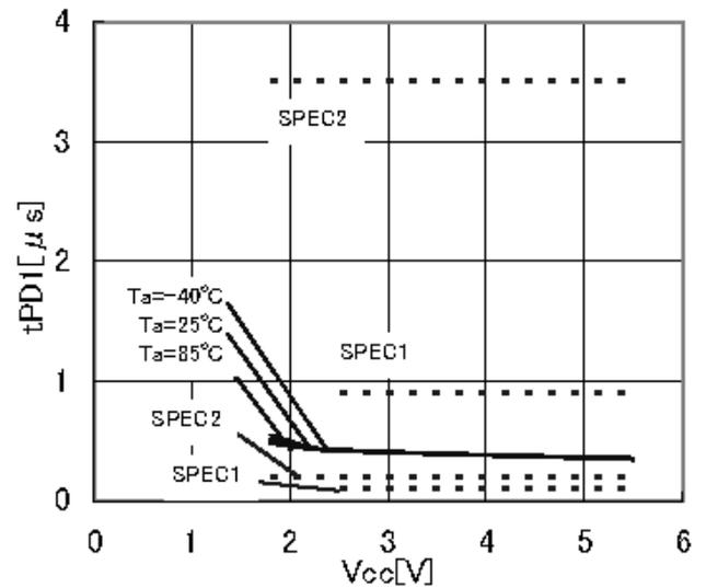
Figure 25. Output data delay time tPD1
