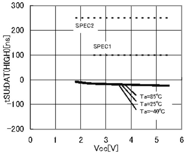
Figure 22. Input data setup time tSU:DAT(HIGH)
