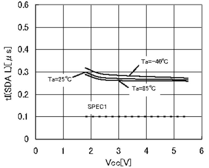
Figure 31. Noise removal valid time  $t_I(\text{SDA L})$
