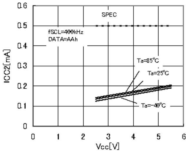
Figure 10. Current consumption at READ action ICC2 (fscL=400kHz)
