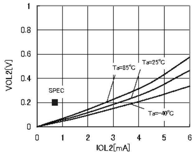
Figure 5. "L" Output Voltage  $V_{OL2}$ - $I_{OL2}$
