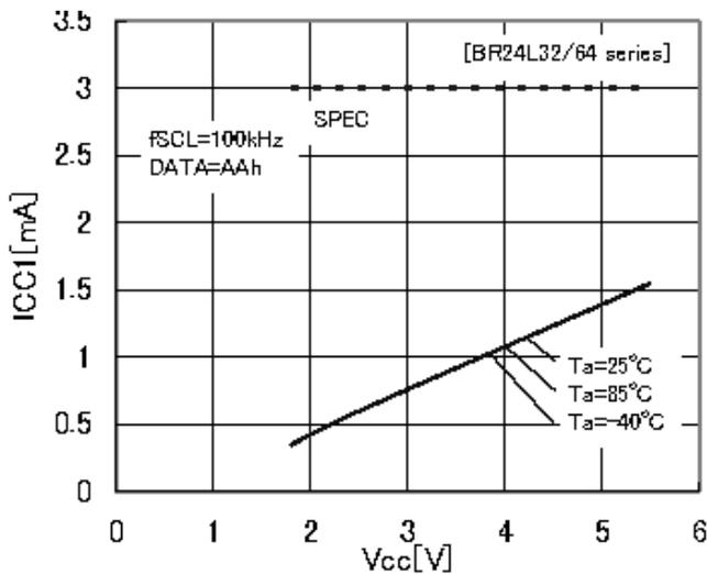
Figure 12. Current consumption at WRITE action ICC1 (fscL=100kHz)
