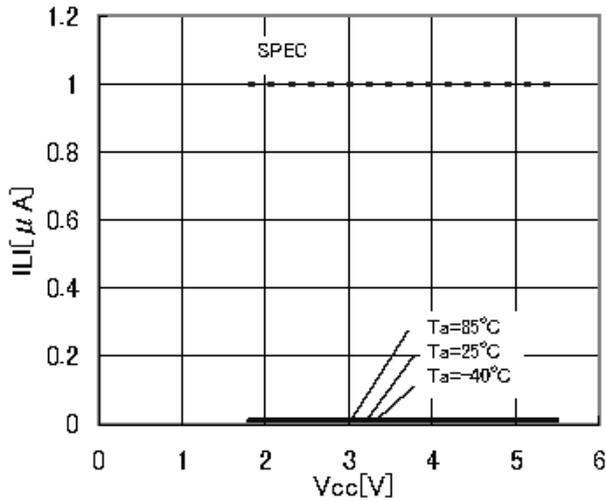
Figure 6. Input Leak Current I<sub>LI</sub> (SCL, WP)
