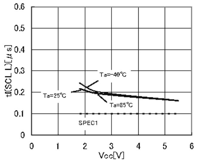
Figure 29. Noise removal valid time tI (SCL L)
