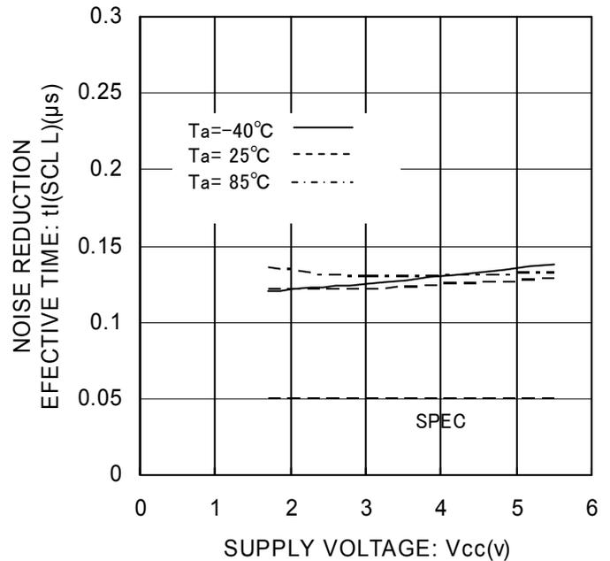
Figure 29. ノイズ除去有効時間  $t_1$ (SCL L)
