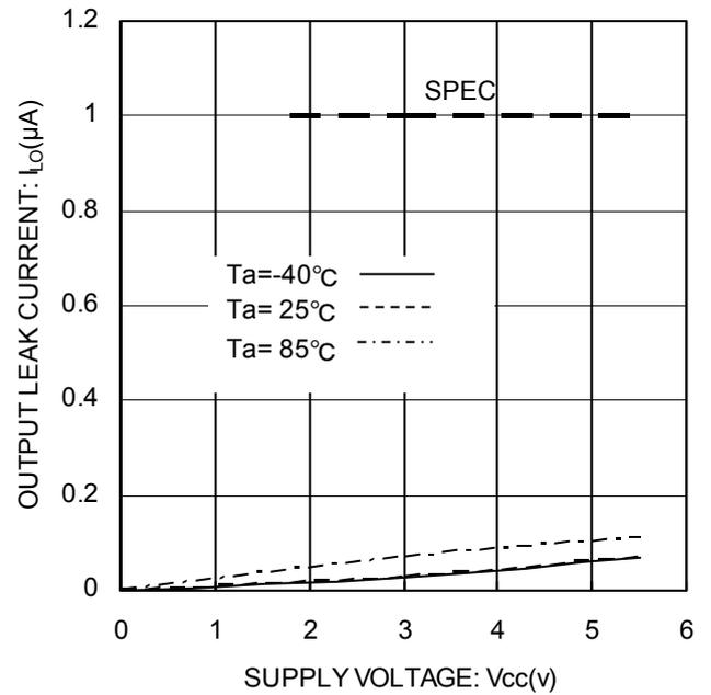
Figure 9. 出力リーク電流  $I_{LO}$  (SDA)
