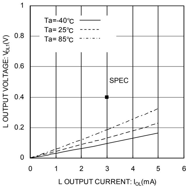
Figure 6. “L”出力電圧  $V_{OL1-I_{OL}}$  ( $V_{CC}=2.5\text{V}$ )
