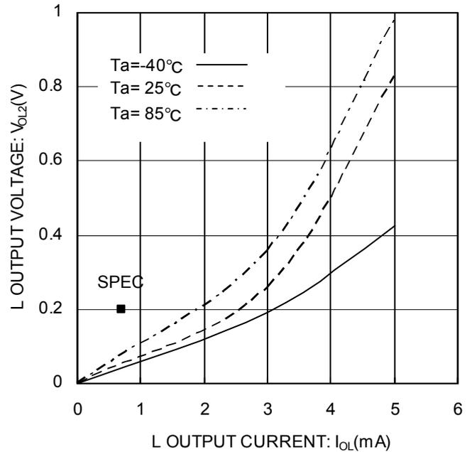
Figure 7. “L”出力電圧  $V_{OL2-I_{OL}}$  ( $V_{CC}=1.7\text{V}$ )
