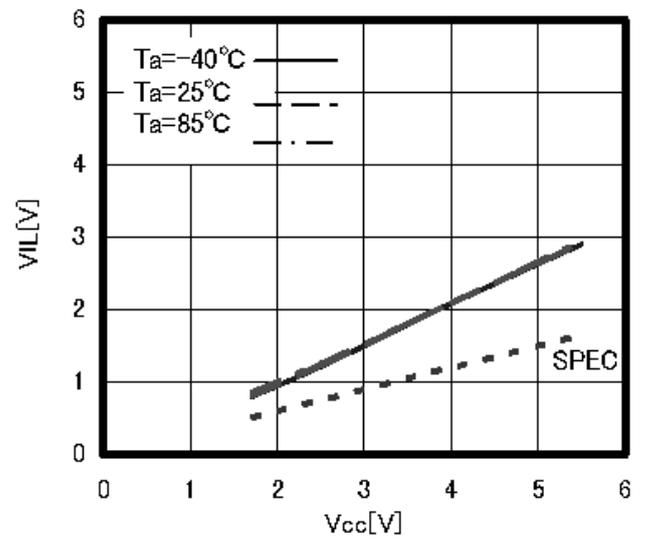
Figure 5. "L" Input Voltage  $V_{IL}$
