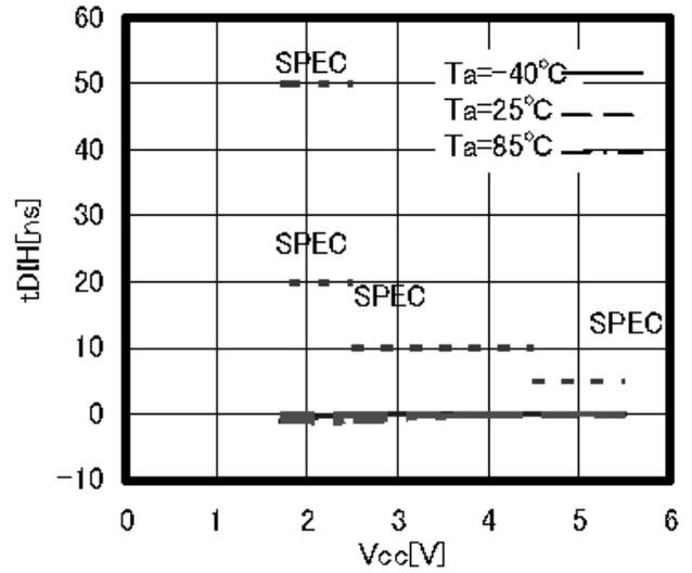
Figure 21. SI hold time  $t_{DIH}$
