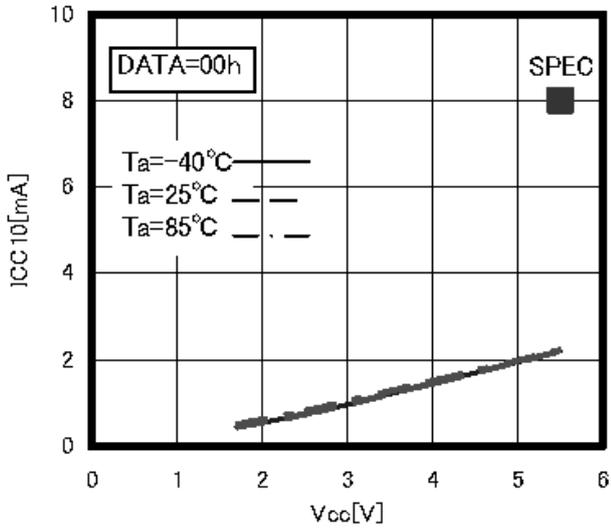
Figure 12. Current consumption at READ operation ICC10
