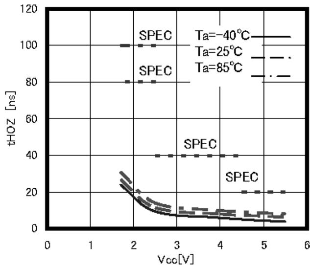
Figure 26. Time from HOLDB to output High-Z tHOZ
