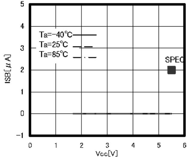
Figure 13. Current consumption at standby operation ISB
