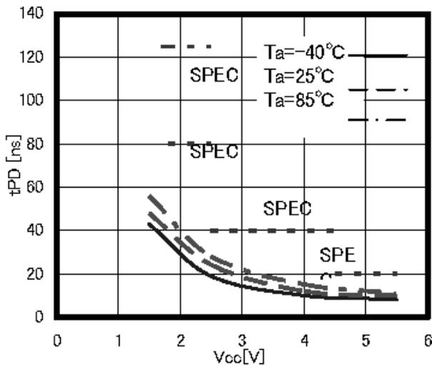
Figure 22. Data output delay time  $t_{PD}$
