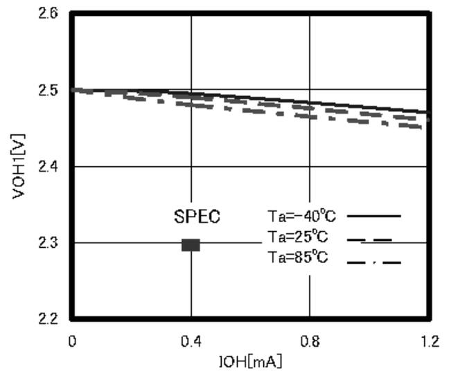
Figure 7. "H" Output Voltage  $V_{OH1}$  ( $V_{CC}=2.5V$ )
