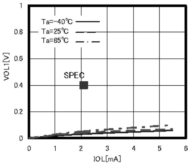
Figure 6. "L" Output Voltage  $V_{OL1}$  ( $V_{CC}=2.5V$ )
