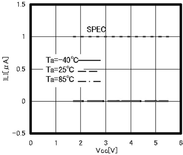
Figure 8. Input Leak Current  $I_{LI}$
