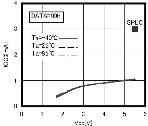
Figure 11. Current consumption at WRITE operation  $ICC3$
