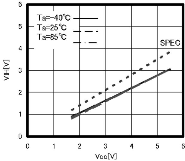
Figure 4. "H" Input Voltage  $V_{IH}$
