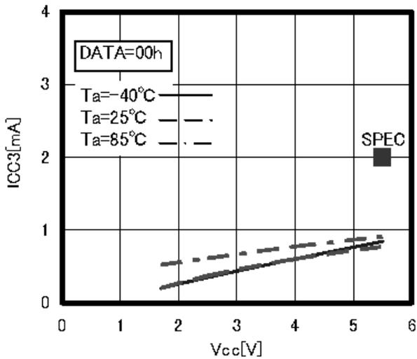
Figure 10. Current consumption at WRITE operation  $ICC3$
