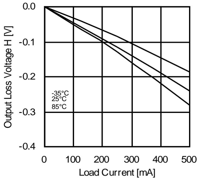
Figure 4. Output Voltage H vs Load Current (BH6578FVM)
