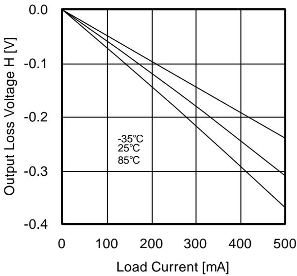
Figure 5. Output Loss Voltage H vs Load Current (BH6578FVM)
