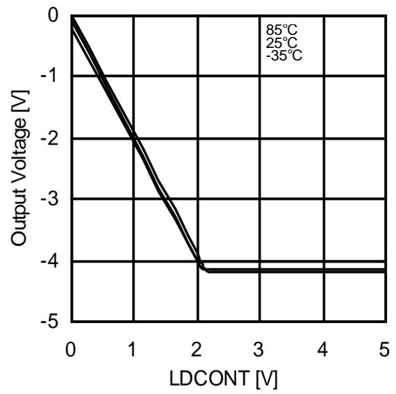
Figure 6. Output Voltage vs Input Voltage (Voltage Gain (BH6578FVM))
