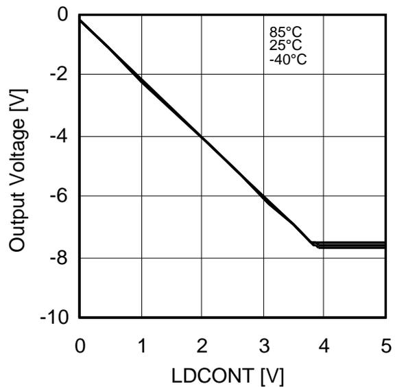
Figure 12. Output Voltage vs Input Voltage (Voltage Gain (BD7931F))
