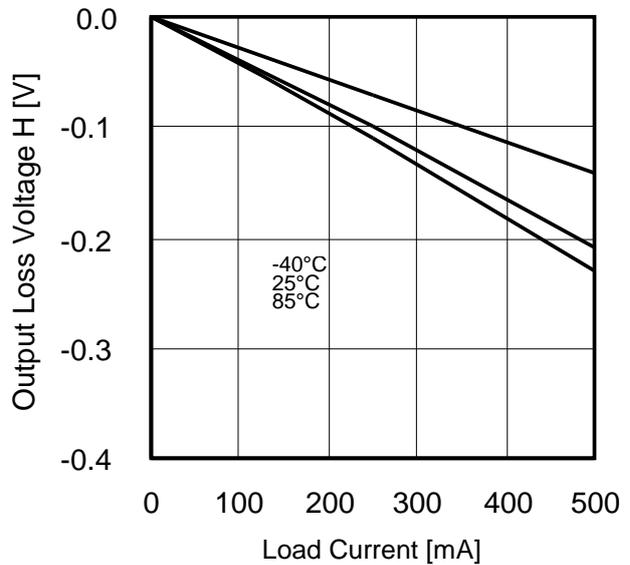
Figure 10. Output Loss Voltage H vs Load Current (BD7931F)
