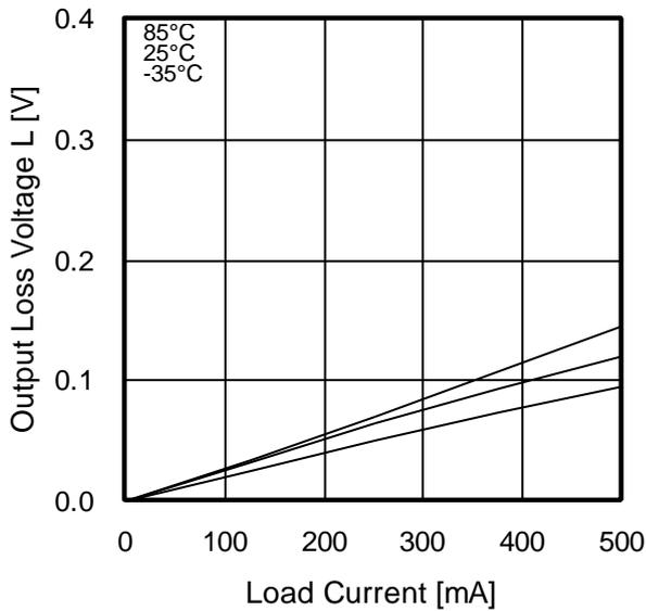
Figure 1. Output Loss Voltage L vs Load Current (BH6578FVM)
