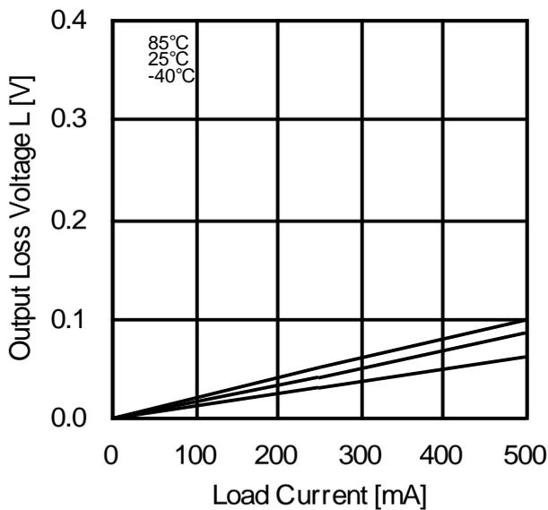
Figure 7. Output Loss Voltage L vs Load Current (BD7931F)
