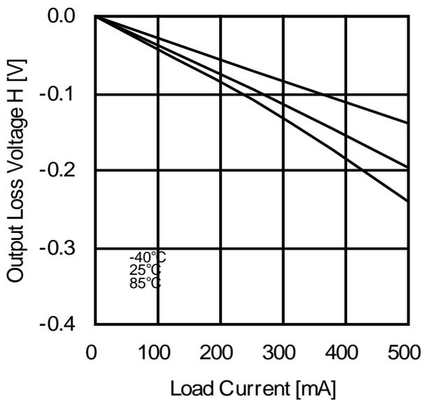
Figure 11. Output Loss Voltage H vs Load Current (BD7931F)
