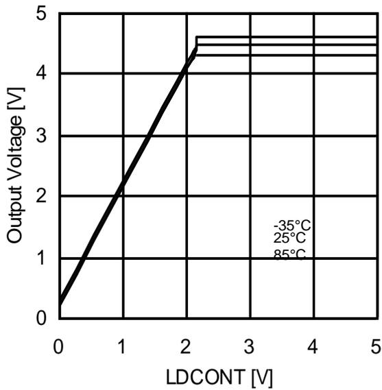
Figure 3. Output Voltage vs Input Voltage (Voltage Gain (BH6578FVM))
