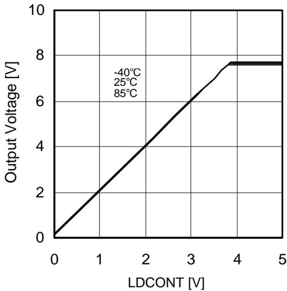
Figure 9. Output Voltage vs Input Voltage (Voltage Gain (BD7931F))
