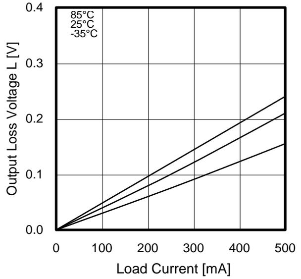
Figure 2. Output Loss Voltage L vs Load Current (BH6578FVM)
