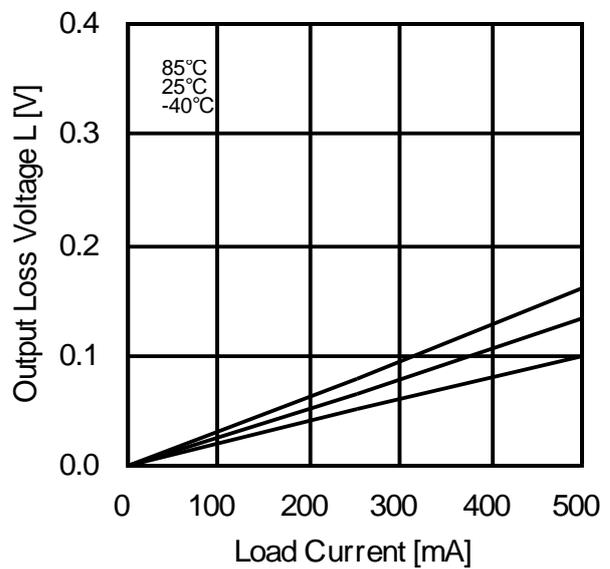
Figure 8. Output Loss Voltage L vs Load Current (BD7931F)
