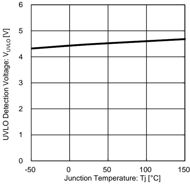
Figure 11. UVLO Detection Voltage vs Junction Temperature
