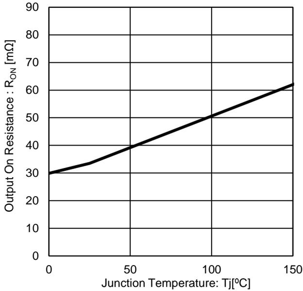
Figure 15. Output ON Resistance vs Junction Temperature
