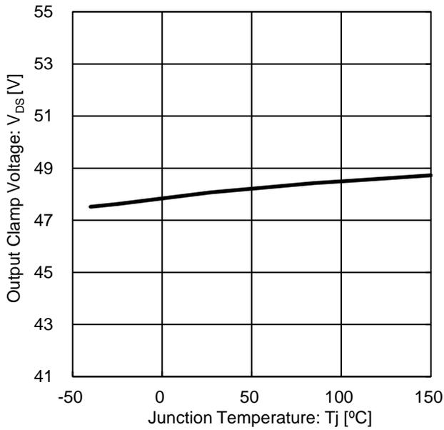
Figure 19. Output Clamp Voltage vs Junction Temperature
