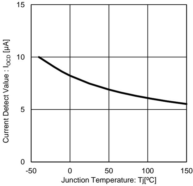
Figure 23. Current Detect Value vs Junction Temperature
