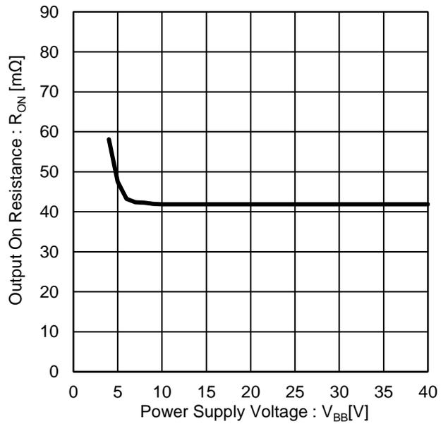
Figure 14. Output ON Resistance vs Supply Voltage
