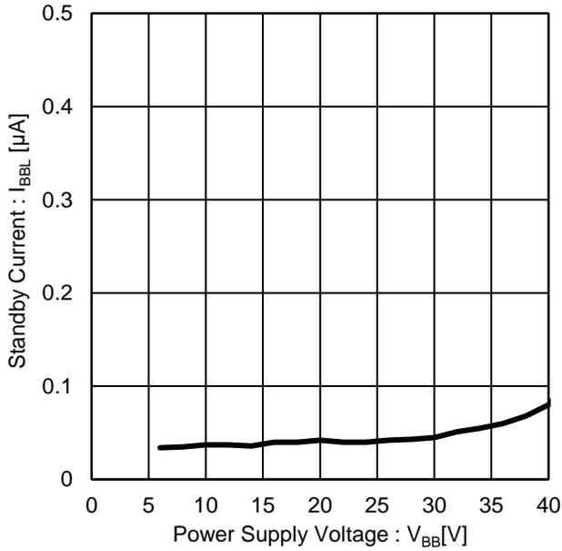
Figure 7. Standby Current vs Power Supply Voltage
