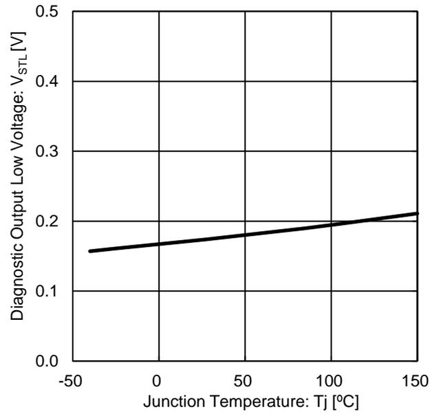
Figure 20. Diagnostic Output Low Voltage vs Junction Temperature
