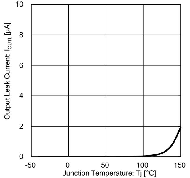
Figure 16. Output leak Current vs Junction Temperature
