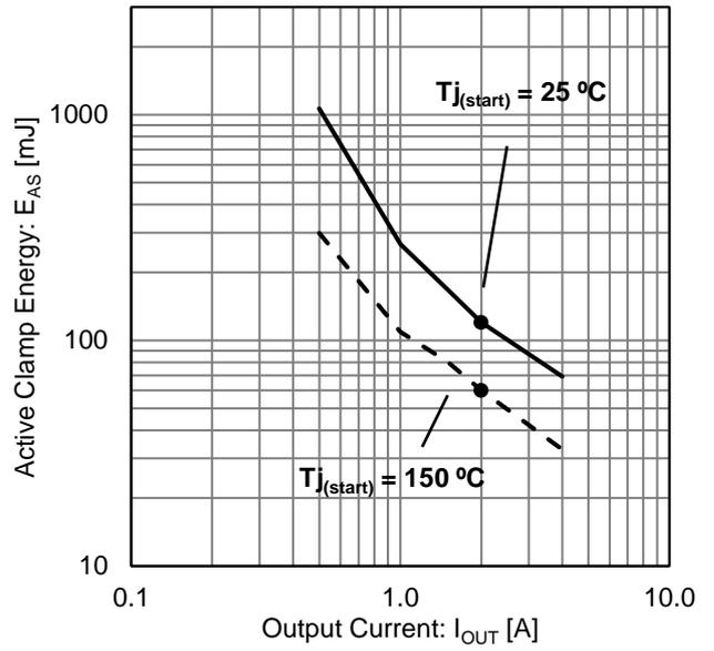
Figure 24. Active Clamp Energy vs Output Current
