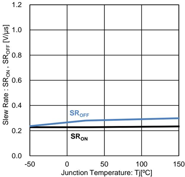
Figure 17. Output Slew Rate vs Junction Temperature
