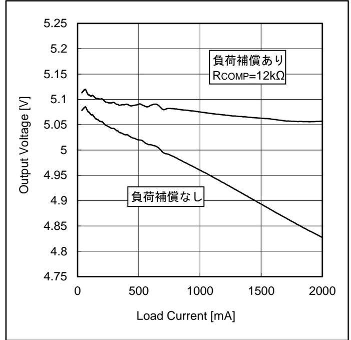
Figure 7. Output Voltage vs Load Current (24V 入力、5V 出力)
