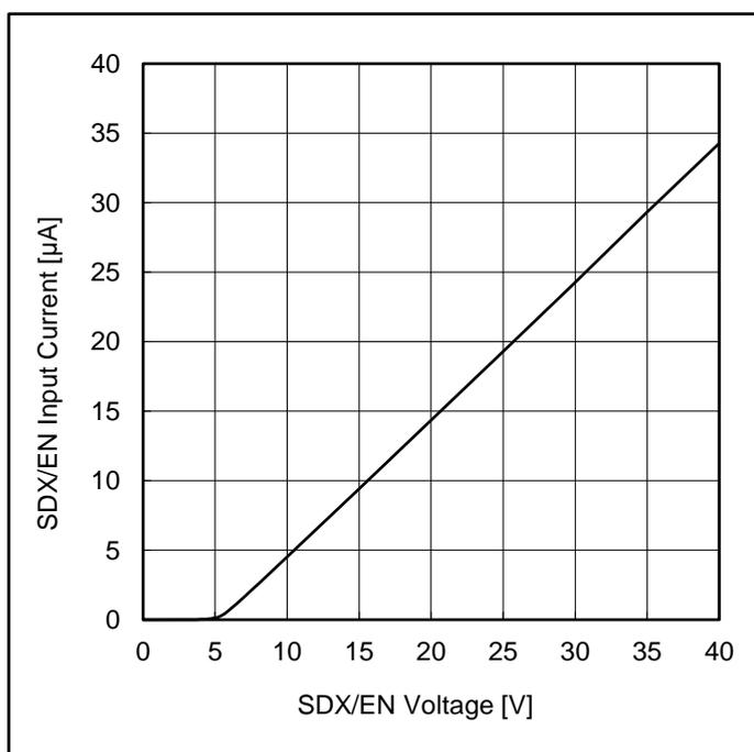
Figure 4. SDX/EN Input Current vs SDX/EN Voltage
