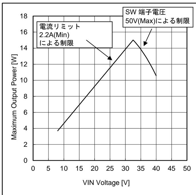
Figure 1. Maximum Output Power vs VIN Voltage
