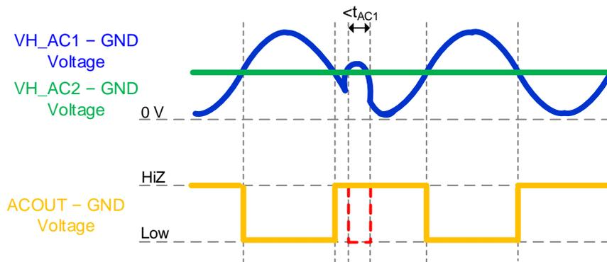
Figure 6. VH\_AC1 and VH\_AC2 Pins Noise Filter 1
