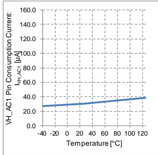
Figure 17. VH\_AC1 Pin Consumption Current vs Temperature
