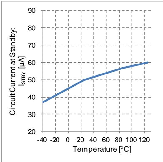
Figure 12. Circuit Current at Standby vs Temperature
