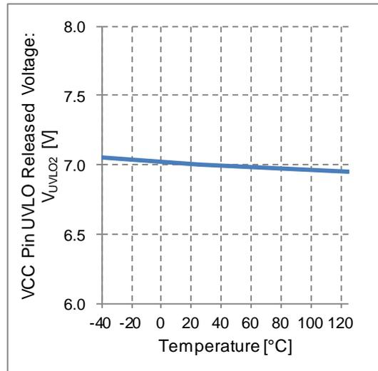
Figure 15. VCC Pin UVLO Released Voltage vs Temperature
