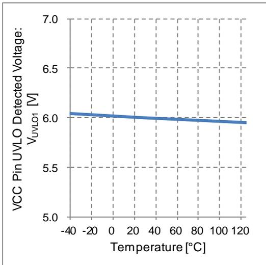
Figure 14. VCC Pin UVLO Detected Voltage vs Temperature
