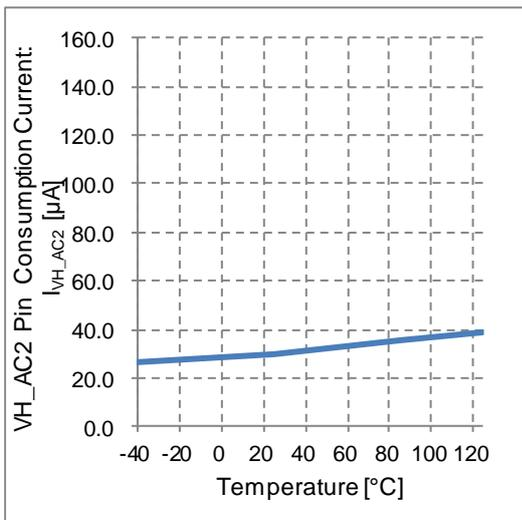
Figure 18. VH\_AC2 Pin Consumption Current vs Temperature
