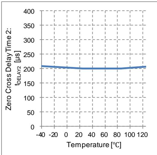
Figure 22. Zero Cross Delay Time 2 vs Temperature
