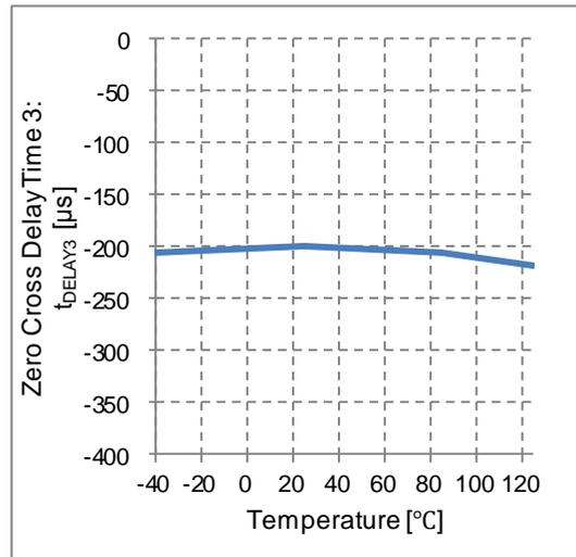
Figure 23. Zero Cross Delay Time 3 vs Temperature
