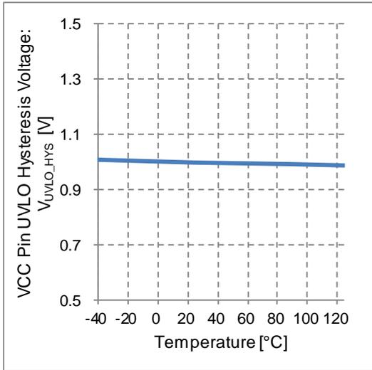
Figure 16. VCC Pin UVLO Hysteresis Voltage vs Temperature
