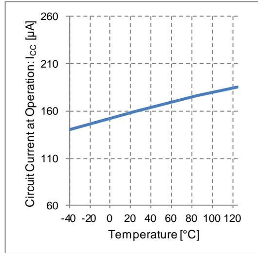
Figure 13. Circuit Current at Operation vs Temperature
