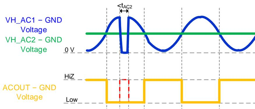
Figure 7. VH\_AC1 and VH\_AC2 Pins Noise Filter 2
