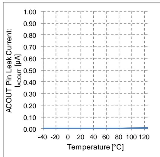
Figure 19. ACOUT Pin Leak Current vs Temperature
