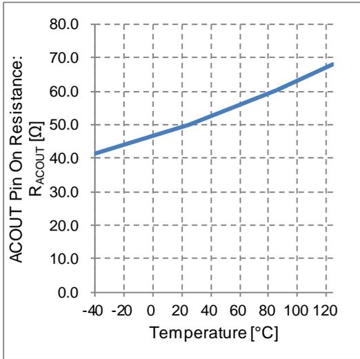
Figure 20. ACOUT Pin On Resistance vs Temperature
