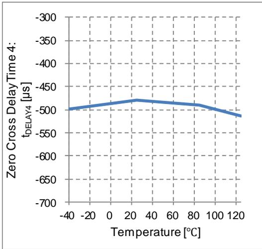
Figure 24. Zero Cross Delay Time 4 vs Temperature
