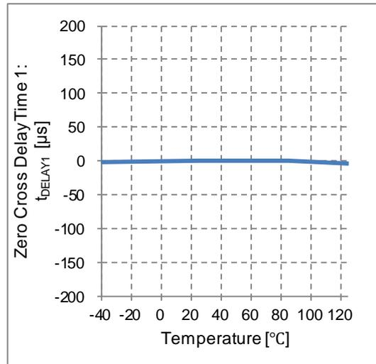
Figure 21. Zero Cross Delay Time 1 vs Temperature
