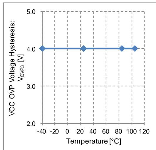
Figure 21. VCC OVP Voltage Hysteresis vs Temperature
