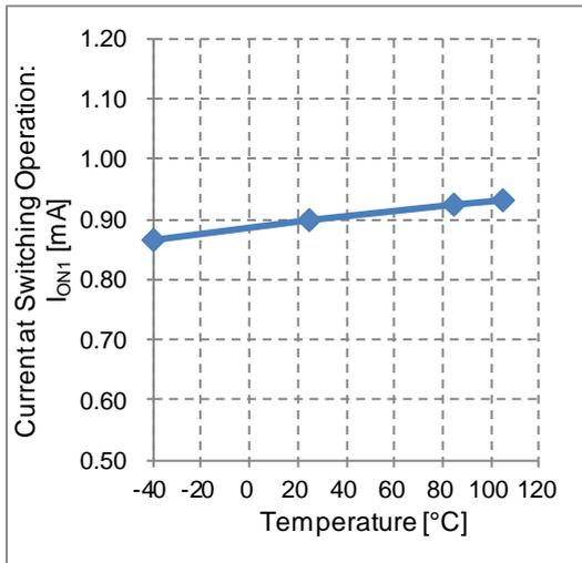
Figure 14. Current at Switching Operation vs Temperature
