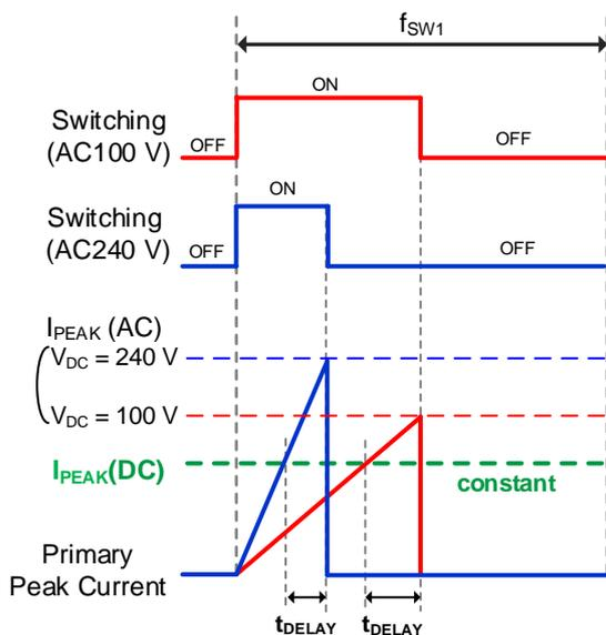
Figure 10. Without the AC Voltage Compensation Function
