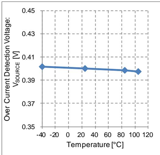
Figure 34. Over Current Detection Voltage vs Temperature
