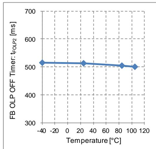
Figure 33. FB OLP OFF Timer vs Temperature
