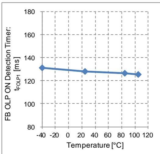
Figure 32. FB OLP ON Detection Timer vs Temperature
