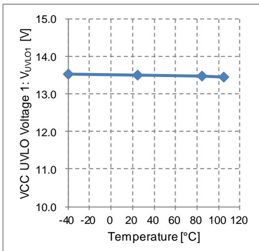
Figure 16. VCC UVLO Voltage 1 vs Temperature
