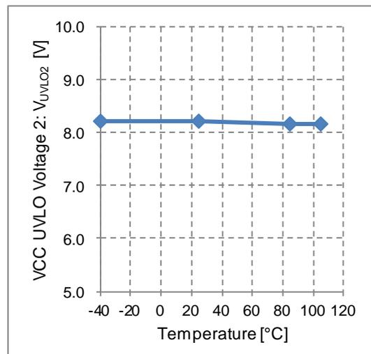
Figure 17. VCC UVLO Voltage 2 vs Temperature
