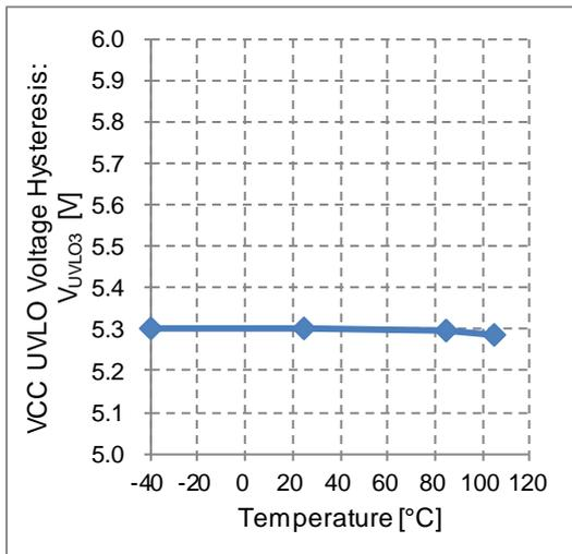
Figure 18. VCC UVLO Voltage Hysteresis vs Temperature
