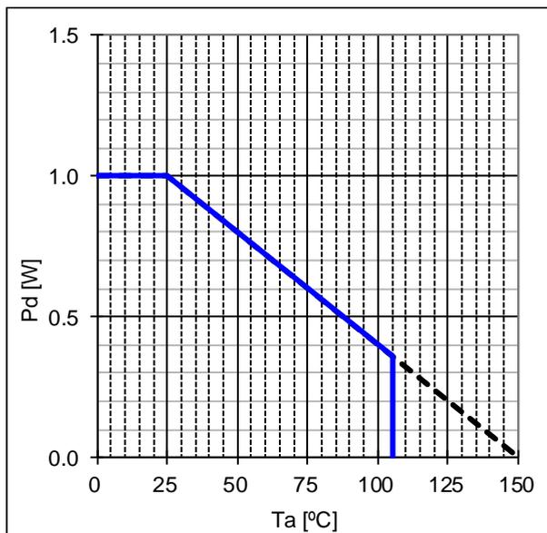
Figure 13. DIP7K Thermal Dissipation Characteristic
