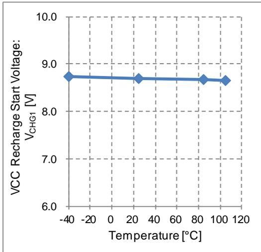
Figure 22. VCC Recharge Start Voltage vs Temperature
