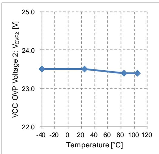
Figure 20. VCC OVP Voltage 2 vs Temperature
