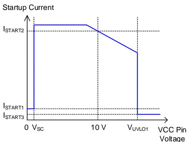
Figure 2. Startup Current vs VCC Pin Voltage
