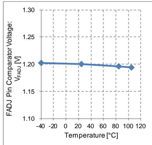
Figure 27. FADJ Pin Comparator Voltage vs Temperature
