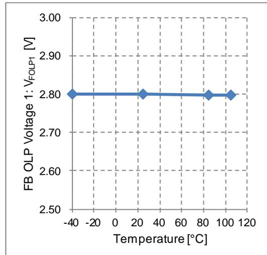
Figure 31. FB OLP Voltage 1 vs Temperature
