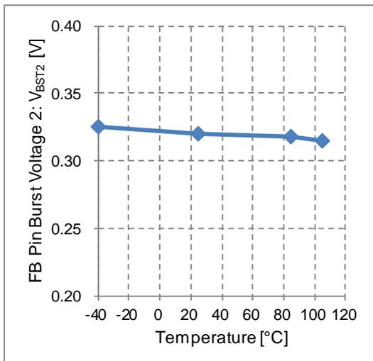
Figure 30. FB Pin Burst Voltage 2 vs Temperature
