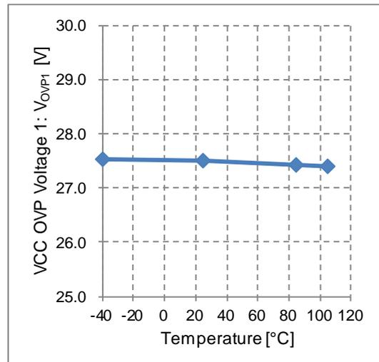
Figure 19. VCC OVP Voltage 1 vs Temperature
