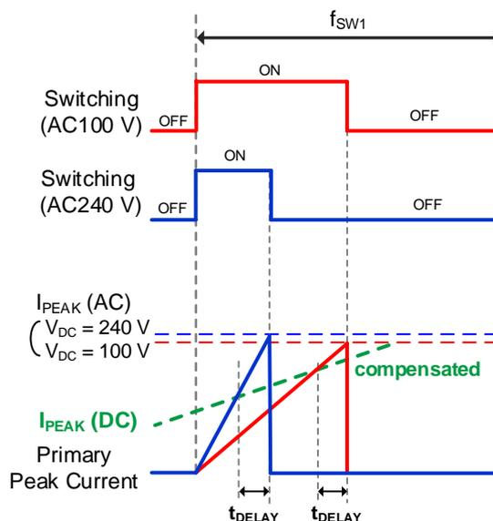
Figure 11. With the AC Voltage Compensation Function
