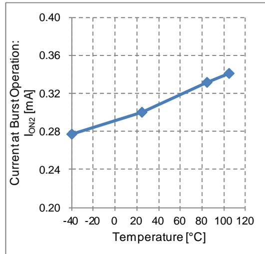
Figure 15. Current at Burst Operation vs Temperature
