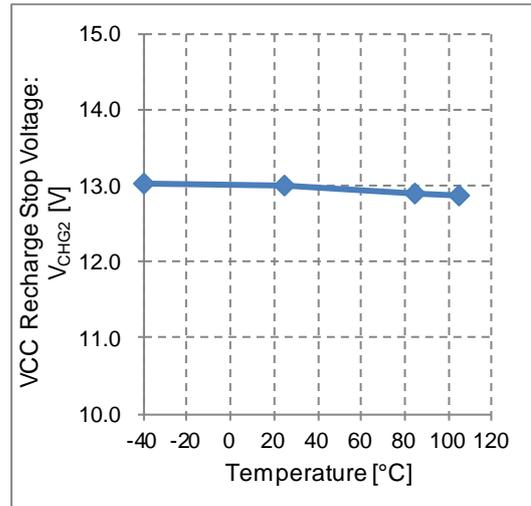
Figure 23. VCC Recharge Stop Voltage vs Temperature
