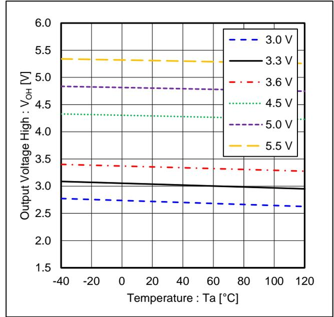
Figure 10. Output Voltage High vs Temperature (@I<sub>SO</sub> = -4 mA)
