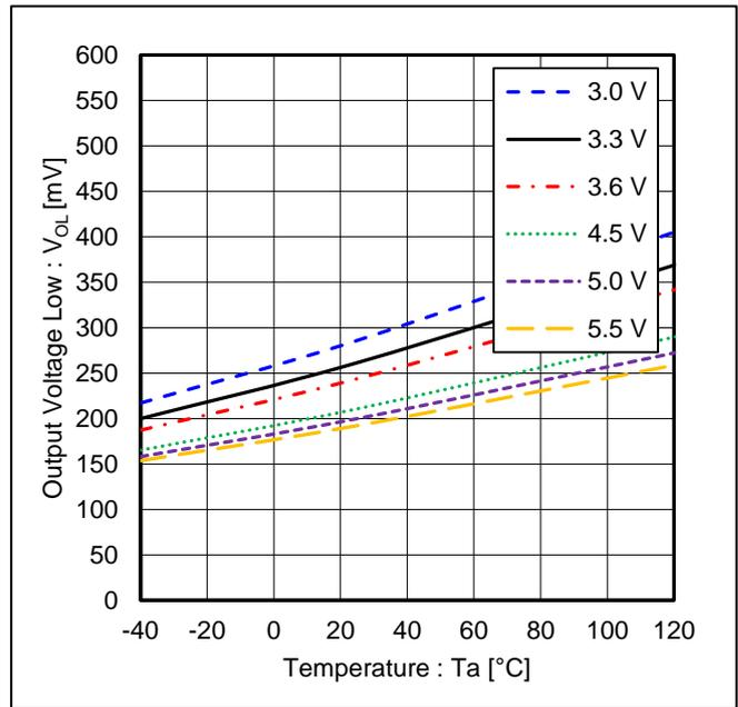
Figure 12. Output Voltage Low vs Temperature (@I<sub>SO</sub> = 4 mA)
