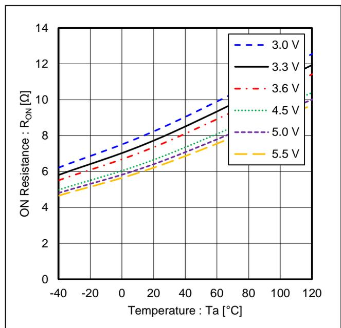
Figure 8. ON Resistance vs Temperature (@IDN = 20 mA)
