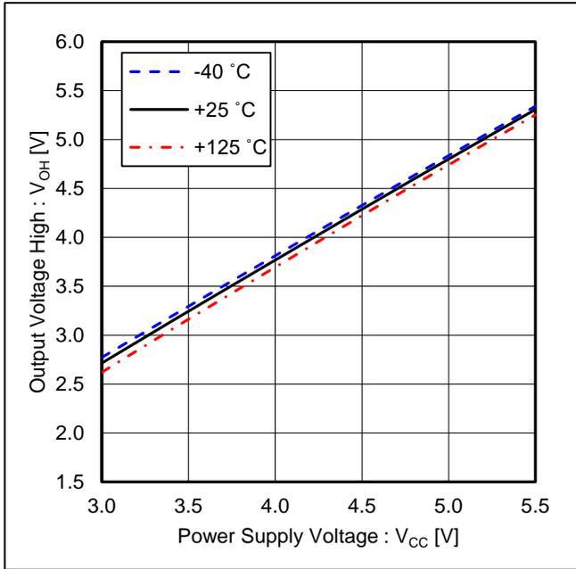
Figure 9. Output Voltage High vs Power Supply Voltage (@I<sub>SO</sub> = -4 mA)
