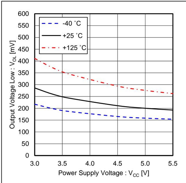
Figure 11. Output Voltage Low vs Power Supply Voltage (@I<sub>SO</sub> = 4 mA)
