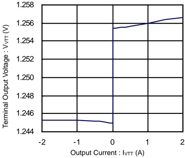
Figure 9. Terminal Output Voltage vs Output Current (DDR-I)
