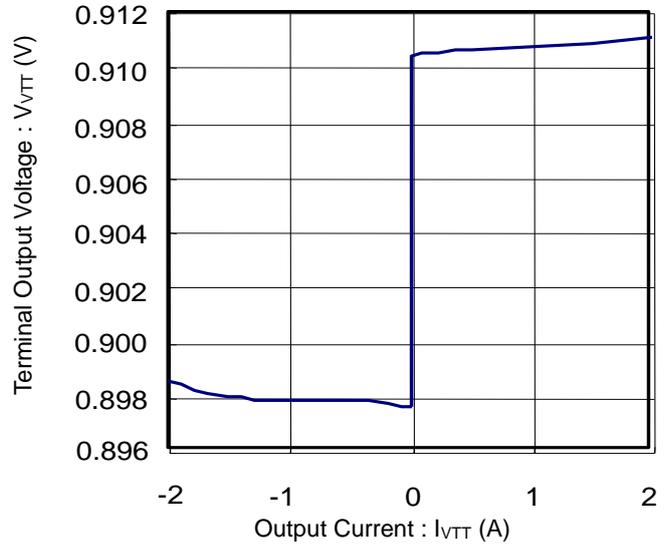
Figure 10. Terminal Output Voltage vs Output Current (DDR-II)
