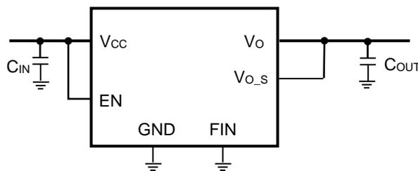
C<sub>IN</sub>, C<sub>OUT</sub>: Ceramic Capacitor
