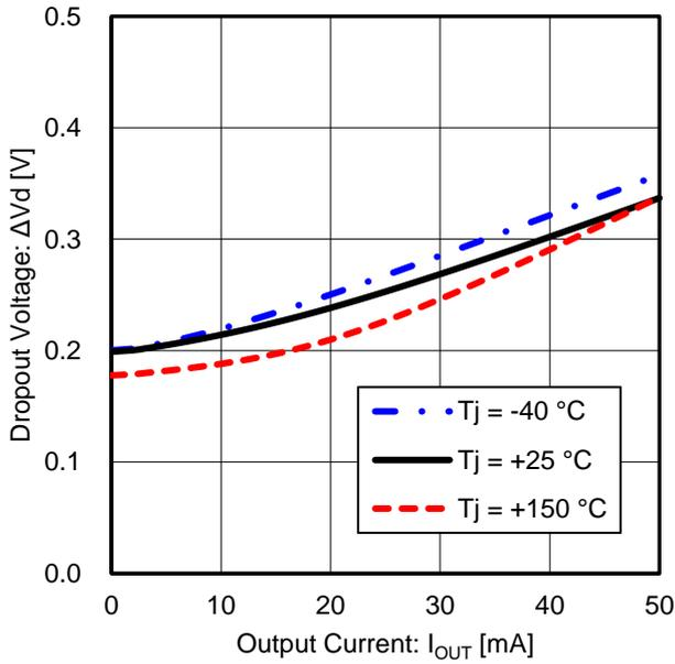
Figure 57. Dropout Voltage vs Output Current
