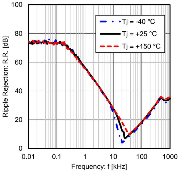
Figure 59. Ripple Rejection vs Frequency
