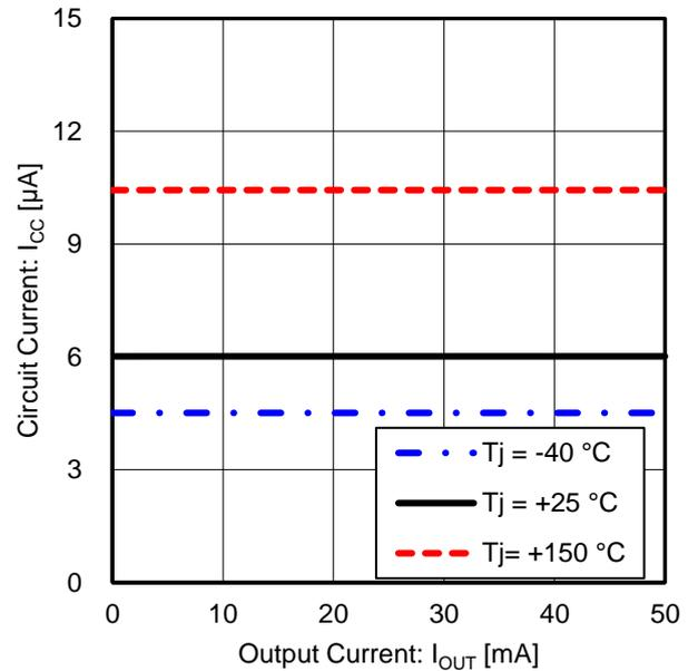
Figure 24. Circuit Current vs Output Current
