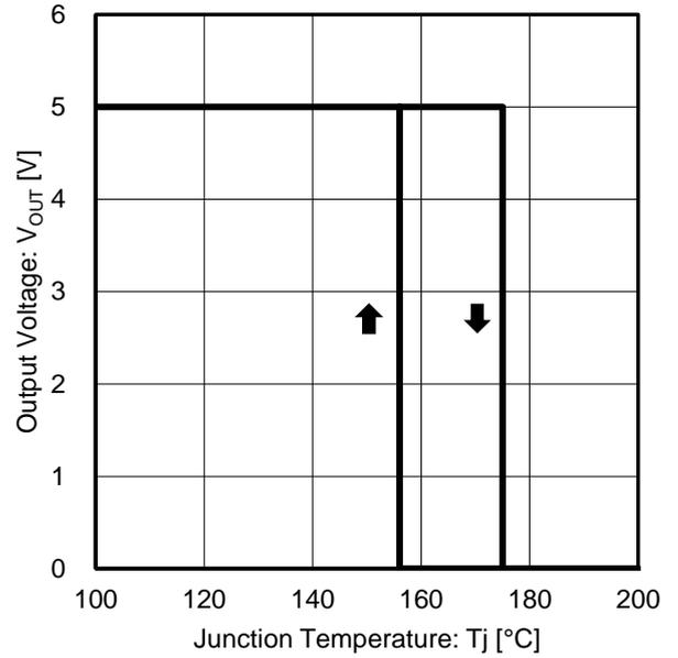
Figure 58. Output Voltage vs Junction Temperature
