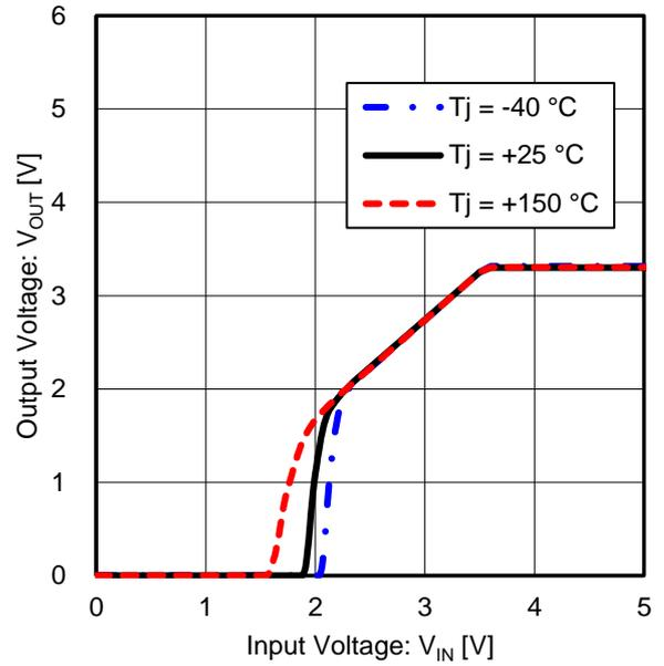
Figure 31. Output Voltage vs Input Voltage - Enlarged view
