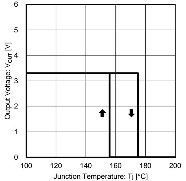
Figure 43. Output Voltage vs Junction Temperature
