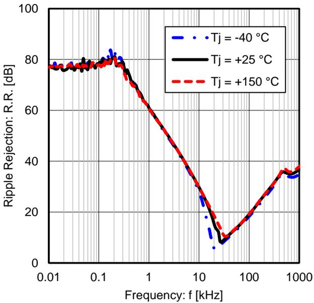
Figure 29. Ripple Rejection vs Frequency
