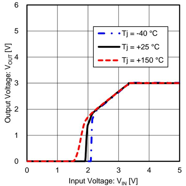
Figure 16. Output Voltage vs Input Voltage - Enlarged view
