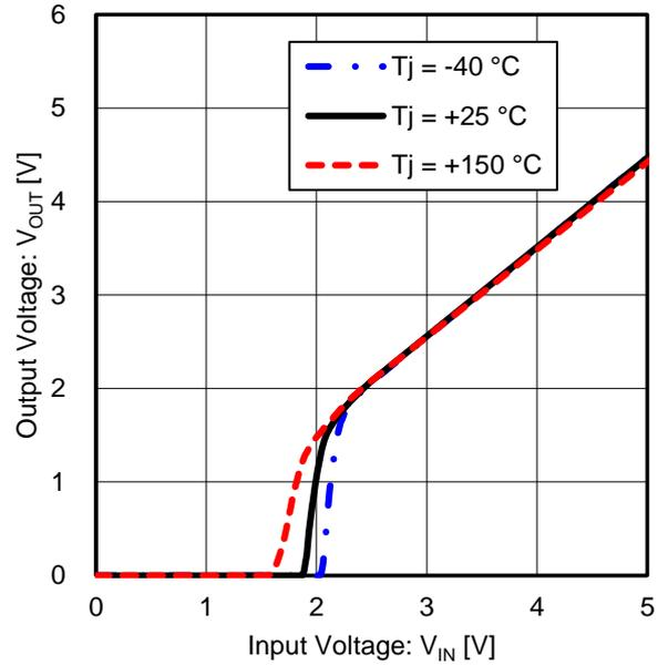
Figure 46. Output Voltage vs Input Voltage - Enlarged view
