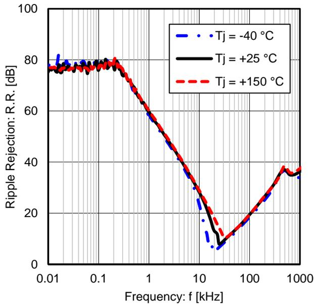
Figure 44. Ripple Rejection vs Frequency
