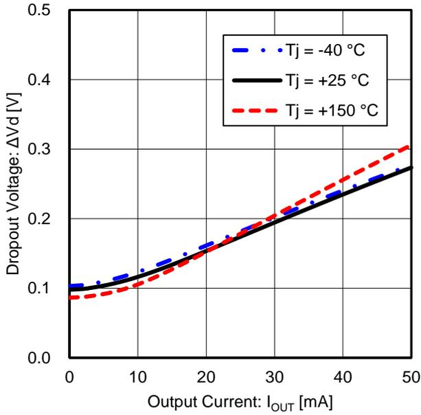
Figure 27. Dropout Voltage vs Output Current
