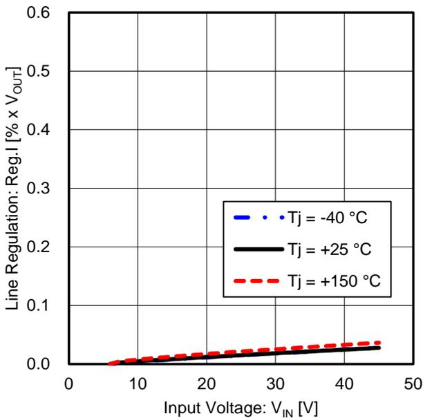
Figure 47. Line Regulation vs Input Voltage
