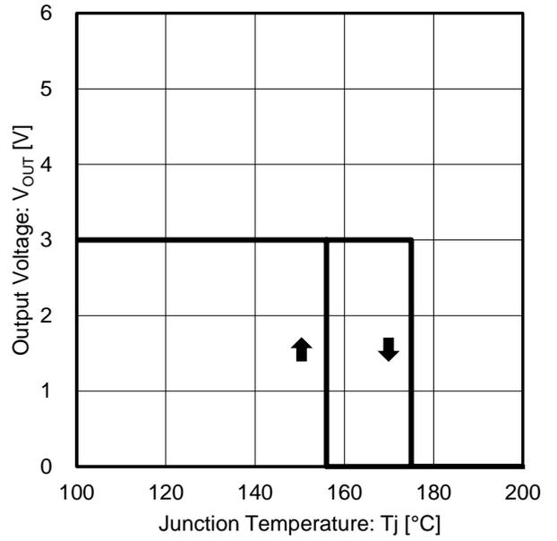
Figure 28. Output Voltage vs Junction Temperature
