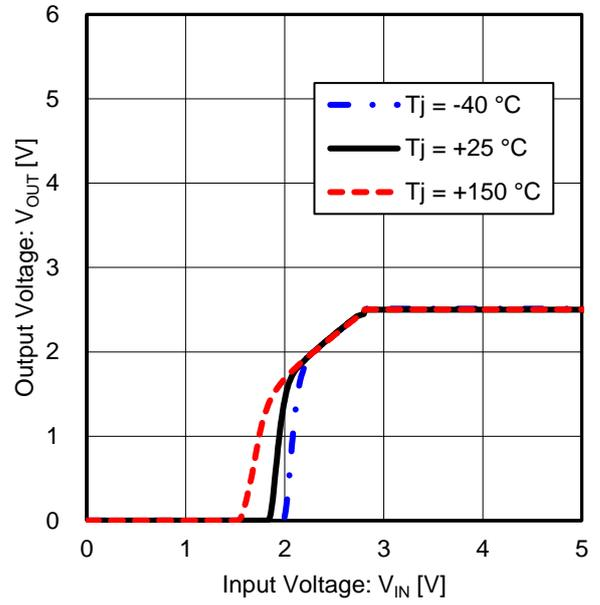
Figure 2. Output Voltage vs Input Voltage - Enlarged view
