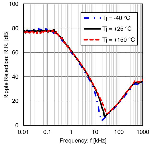
Figure 14. Ripple Rejection vs Frequency ( $I_{OUT} = 50\text{ mA}$ )
