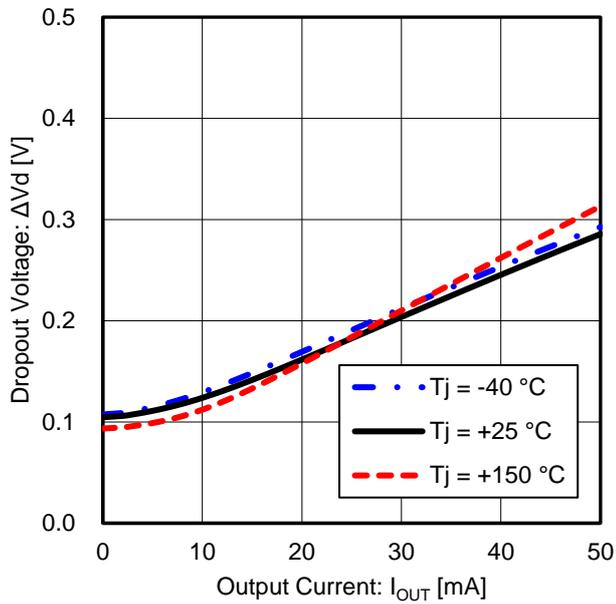
Figure 42. Dropout Voltage vs Output Current
