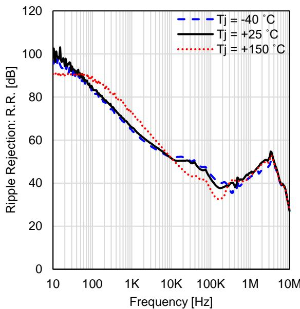
Figure 38. Ripple Rejection vs Frequency
