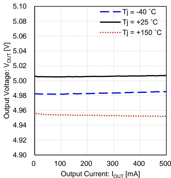
Figure 12. Output Voltage vs Output Current
