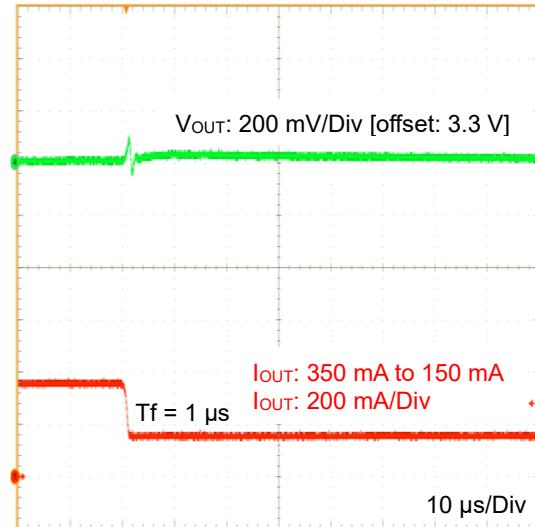
Figure 46. Load Transient 350 mA to 150 mA
