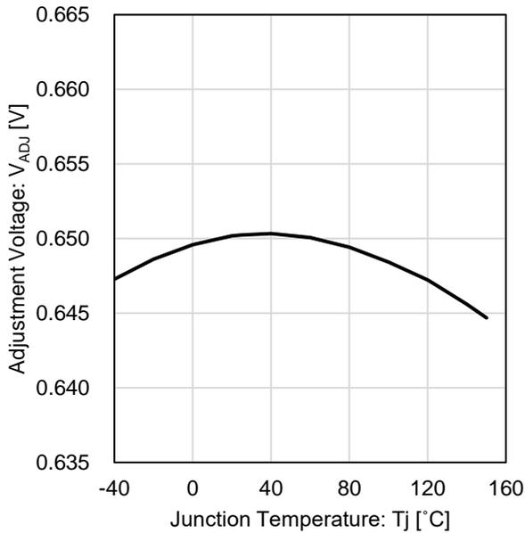
Figure 15. Adjustment Voltage vs Junction Temperature
