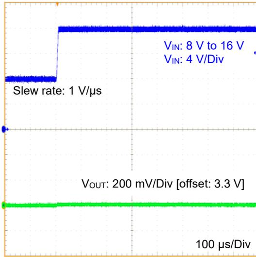
Figure 47. Line Transient 8 V to 16 V
