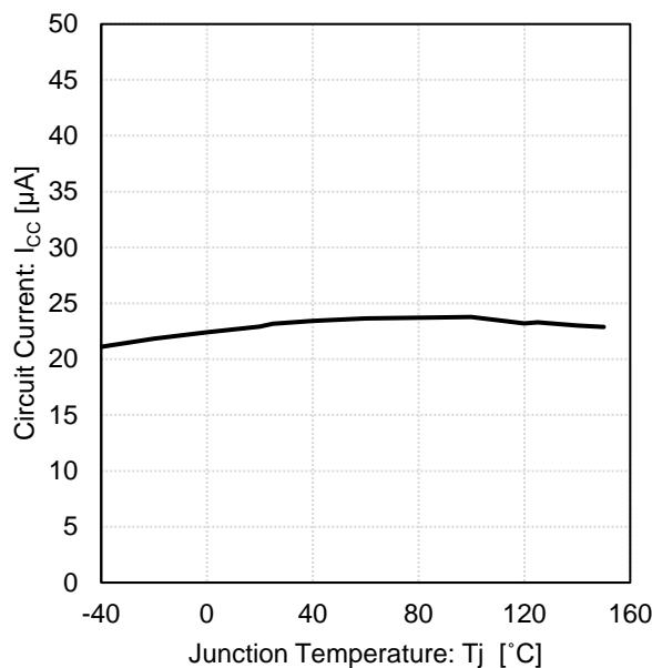
Figure 35. Circuit Current vs Junction Temperature
