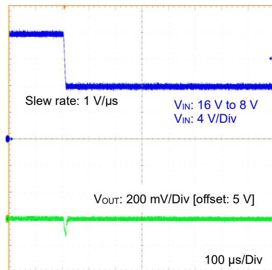
Figure 26. Line Transient 16 V to 8 V
