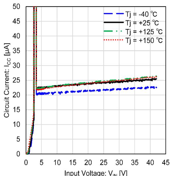
Figure 32. Circuit Current vs Input Voltage;
