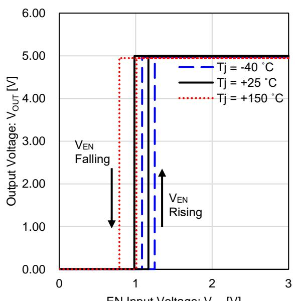
Figure 18. Output Voltage vs EN Input Voltage
