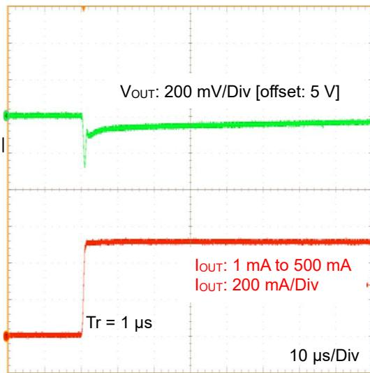
Figure 19. Load Transient 1 mA to 500 mA
