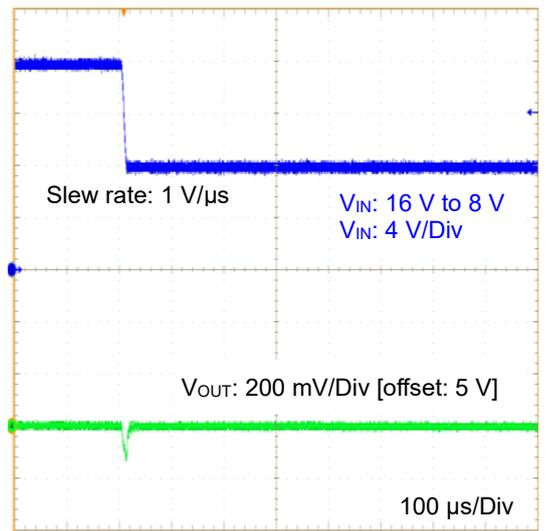
Figure 26. Line Transient 16 V to 8 V
