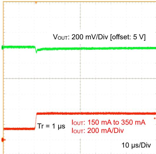
Figure 21. Load Transient 150 mA to 350 mA
