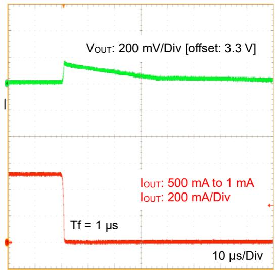
Figure 44. Load Transient 500 mA to 1 mA
