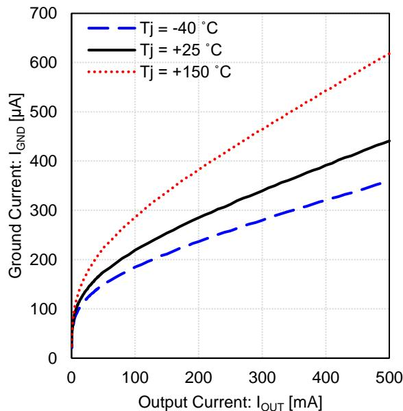
Figure 3. Ground Current vs Output Current
