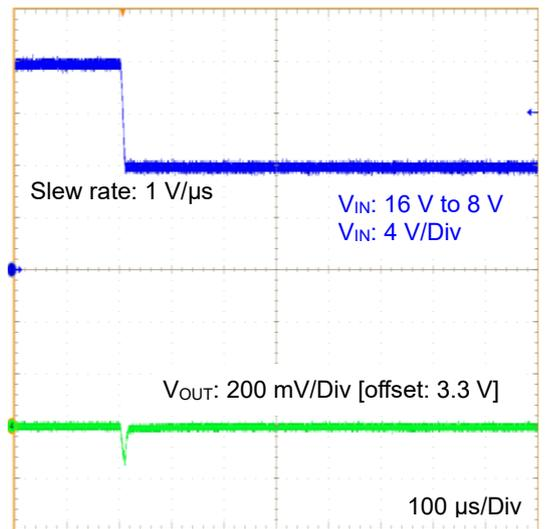
Figure 50. Line Transient 16 V to 8 V
