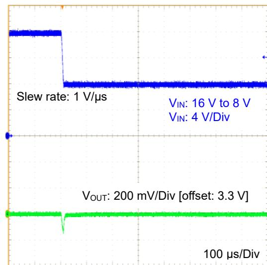
Figure 50. Line Transient 16 V to 8 V
