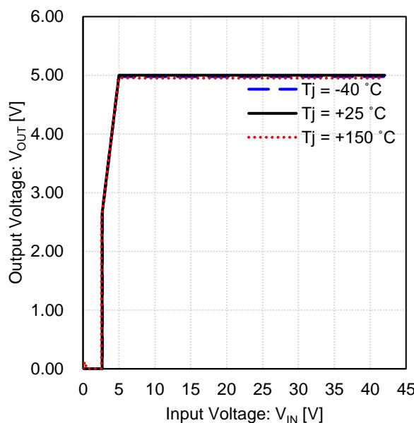
Figure 9. Output Voltage vs Input Voltage
