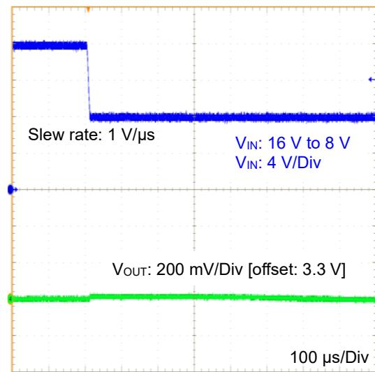
Figure 48. Line Transient 16 V to 8 V
