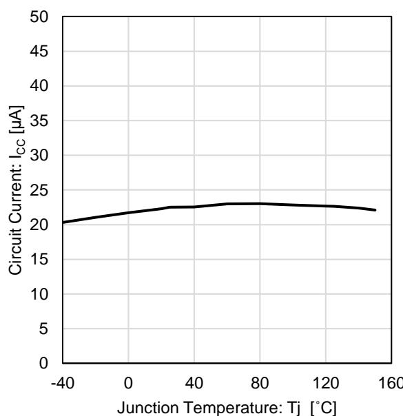
Figure 5. Circuit Current vs Junction Temperature
