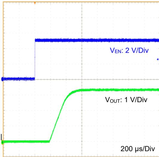
Figure 53. EN Startup Waveform
