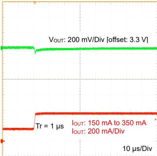
Figure 45. Load Transient 150 mA to 350 mA
