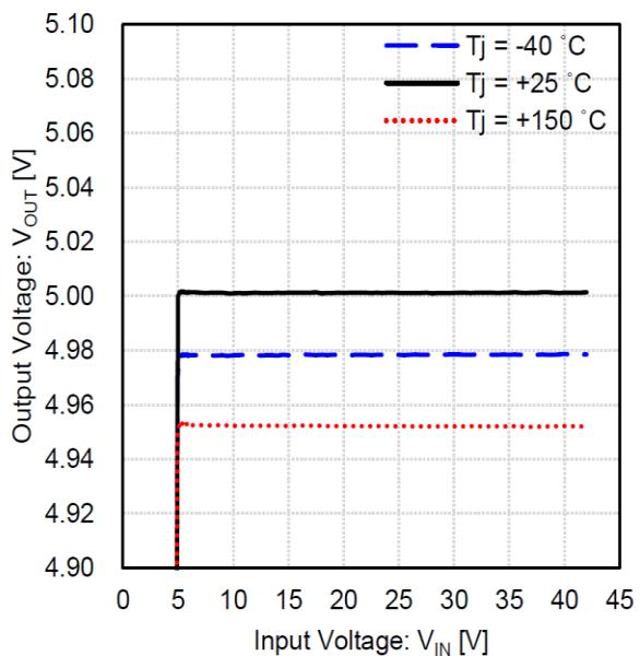
Figure 10. Output Voltage vs Input Voltage;
