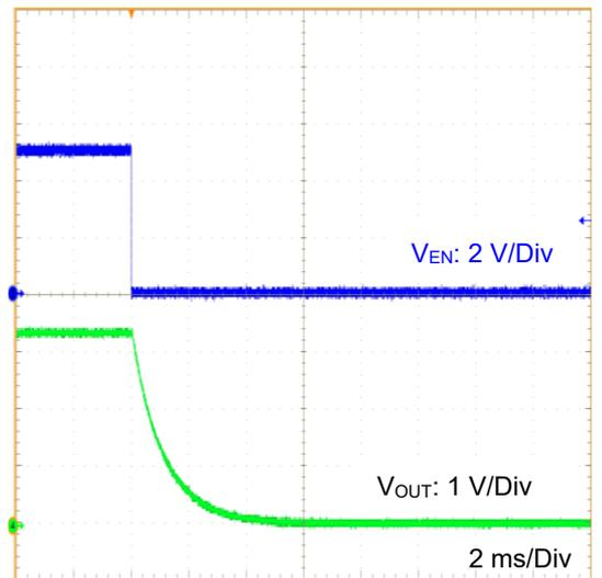
Figure 54. EN Shutdown Waveform
