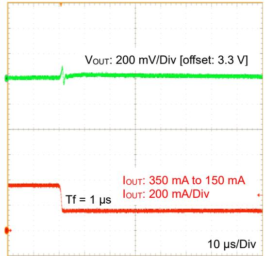
Figure 46. Load Transient 350 mA to 150 mA
