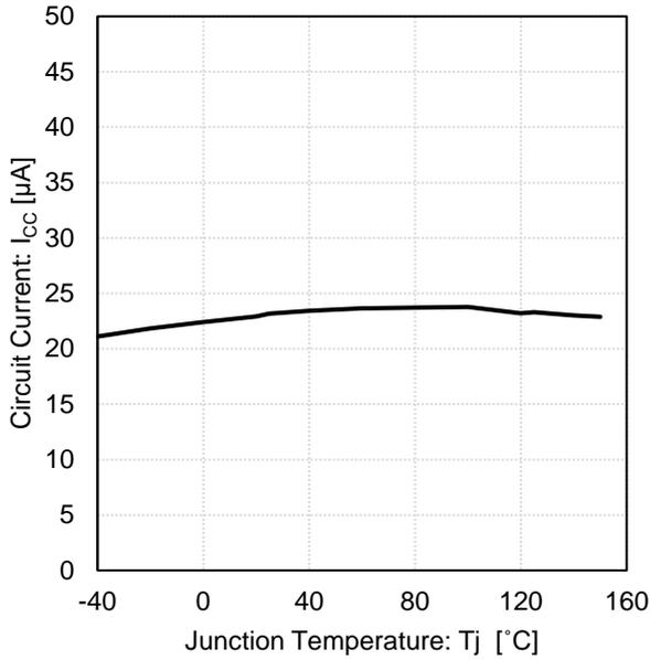
Figure 35. Circuit Current vs Junction Temperature (3.3 V output)
