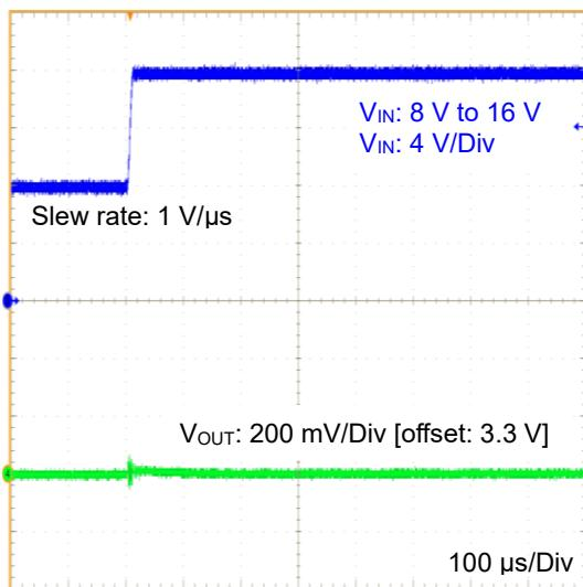
Figure 49. Line Transient 8 V to 16 V
