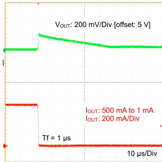
Figure 20. Load Transient 500 mA to 1 mA
