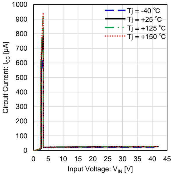
Figure 31. Circuit Current vs Input Voltage (3.3 V output)
