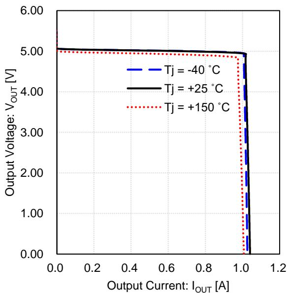
Figure 13. Output Voltage vs Output Current
