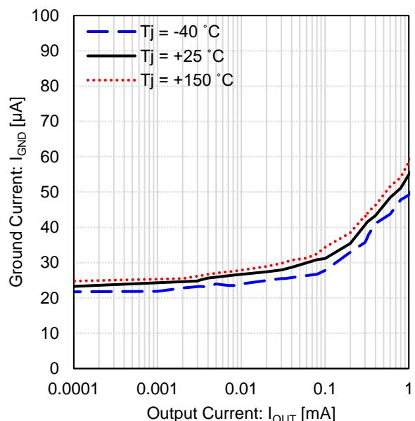
Figure 34. Ground Current vs Output Current;
