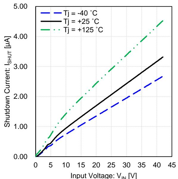
Figure 16. Shutdown Current vs Input Voltage
