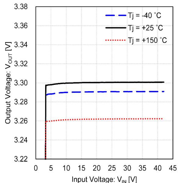
Figure 40. Output Voltage vs Input Voltage;
