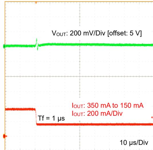
Figure 22. Load Transient 350 mA to 150 mA
