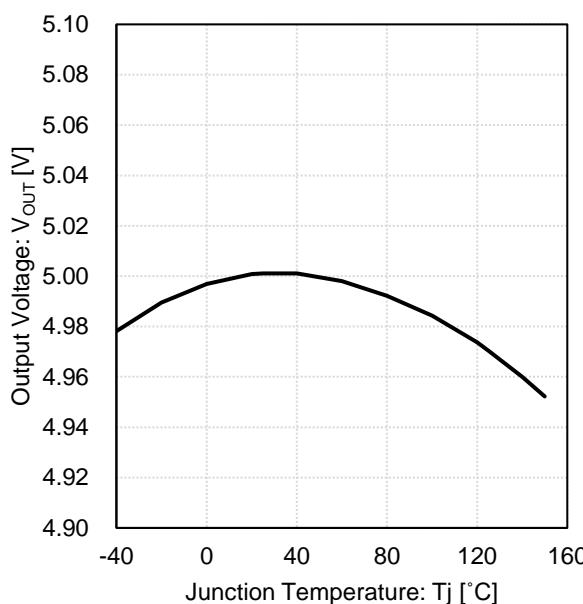
Figure 6. Output Voltage vs Junction Temperature
