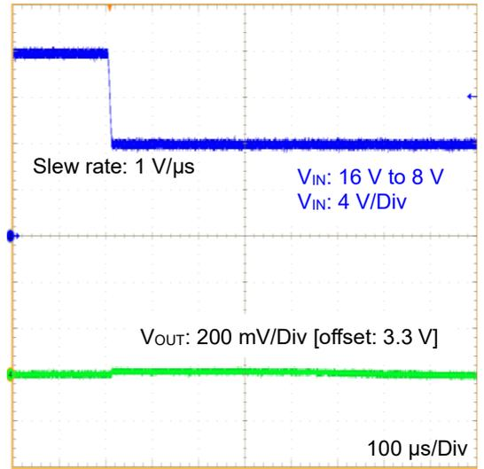
Figure 48. Line Transient 16 V to 8 V
