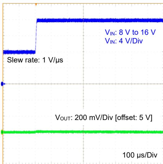
Figure 23. Line Transient 8 V to 16 V
