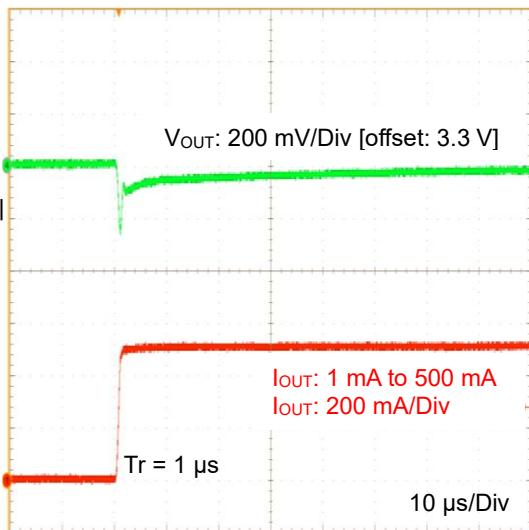
Figure 43. Load Transient 1 mA to 500 mA
