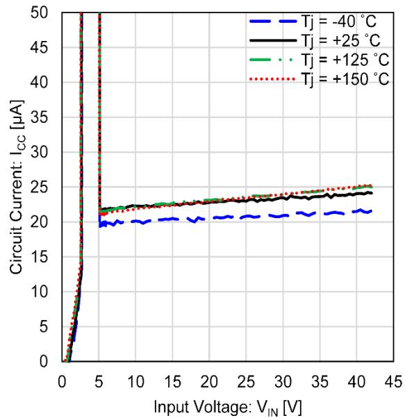
Figure 2. Circuit Current vs Input Voltage;
