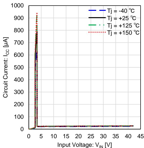
Figure 31. Circuit Current vs Input Voltage
