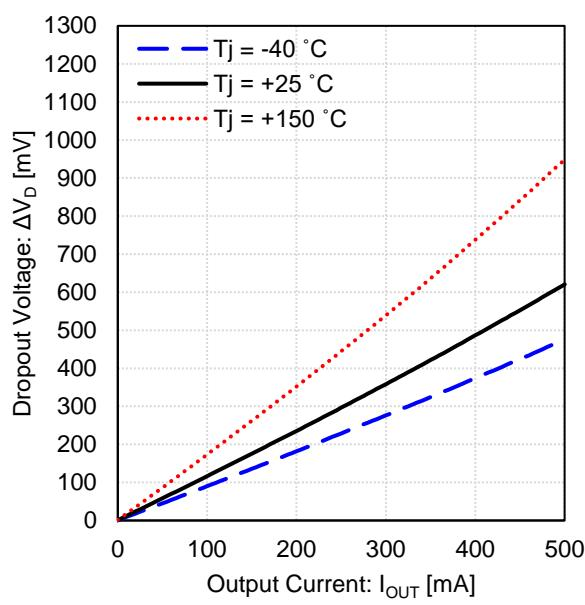
Figure 7. Dropout Voltage vs Output Current
