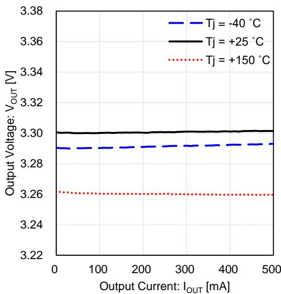
Figure 41. Output Voltage vs Output Current
