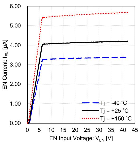
Figure 17. EN Bias Current vs EN Input Voltage
