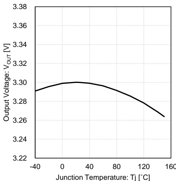
Figure 36. Output Voltage vs Junction Temperature
