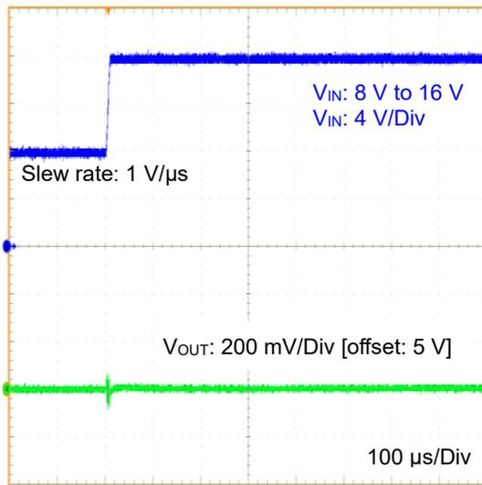
Figure 25. Line Transient 8 V to 16 V
