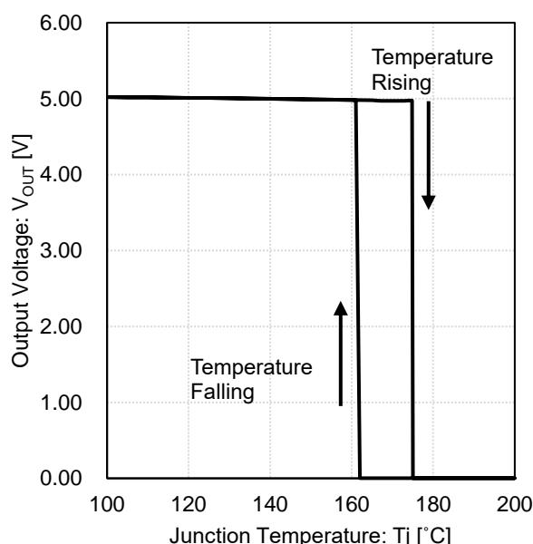
Figure 14. Output Voltage vs Junction Temperature
