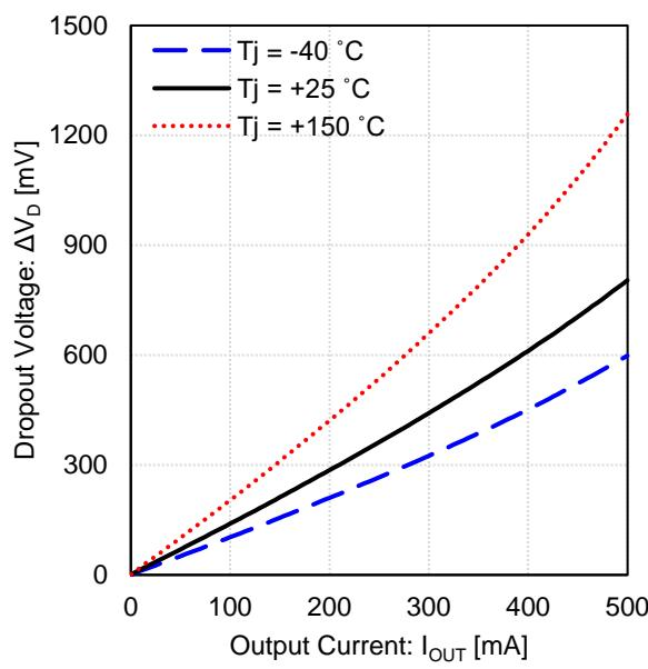
Figure 37. Dropout Voltage vs Output Current
