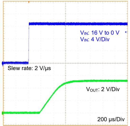
Figure 52. VIN Startup Waveform
