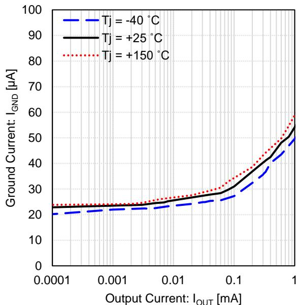
Figure 4. Ground Current vs Output Current;
