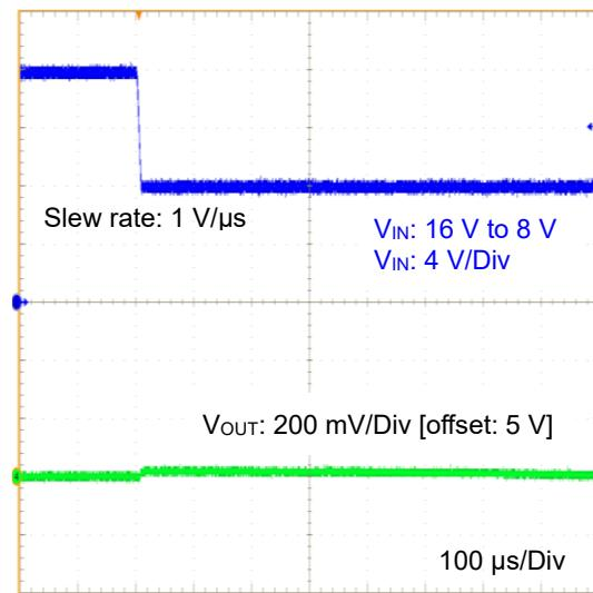
Figure 24. Line Transient 16 V to 8 V
