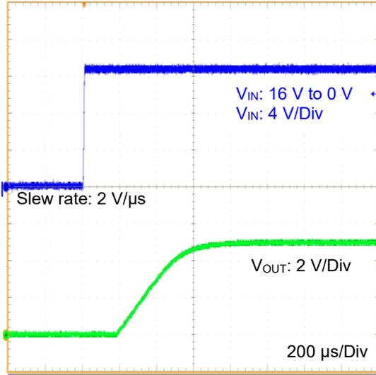
Figure 51. VIN Startup Waveform
