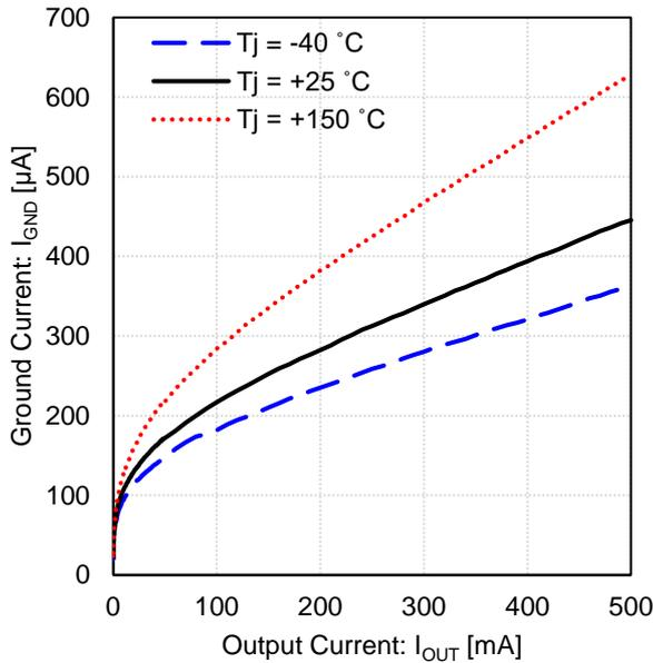
Figure 33. Ground Current vs Output Current (3.3 V output)
