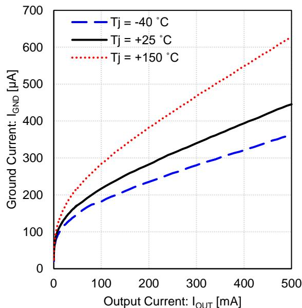
Figure 33. Ground Current vs Output Current
