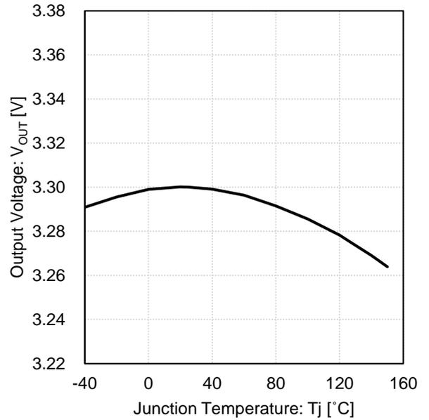
Figure 36. Output Voltage vs Junction Temperature (3.3 V output)
