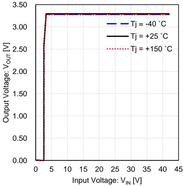
Figure 39. Output Voltage vs Input Voltage (3.3 V output)
