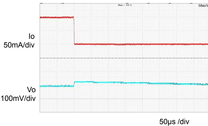
Figure 11. 過渡応答 ( T_a=-40^\circ\text{C} ) ( I_o = 0.1\text{A} \rightarrow 0\text{A} )
