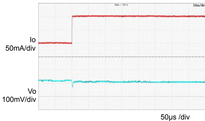
Figure 8. 過渡応答 ( T_a=25^\circ\text{C} ) ( I_o = 0\text{A}\rightarrow 0.1\text{A} )
