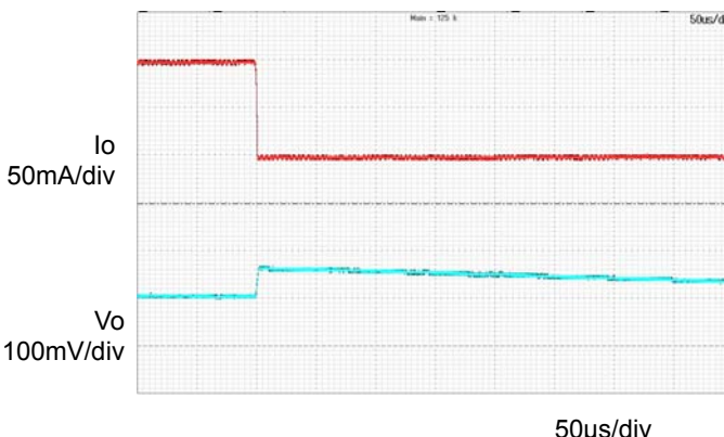
Figure 13. 過渡応答 ( T_a=105^\circ\text{C} ) ( I_o = 0.1\text{A} \rightarrow 0\text{A} )
