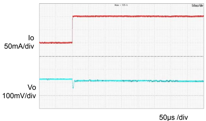
Figure 12. 過渡応答 ( T_a=105^\circ\text{C} ) ( I_o = 0\text{A} \rightarrow 0.1\text{A} )
