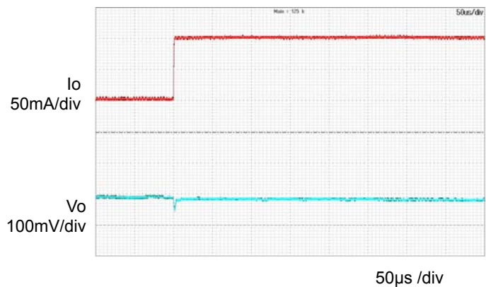
Figure 10. 過渡応答 ( T_a=-40^\circ\text{C} ) ( I_o = 0\text{A} \rightarrow 0.1\text{A} )
