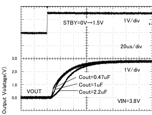
Figure 42. Startup time ( Rout = none )
