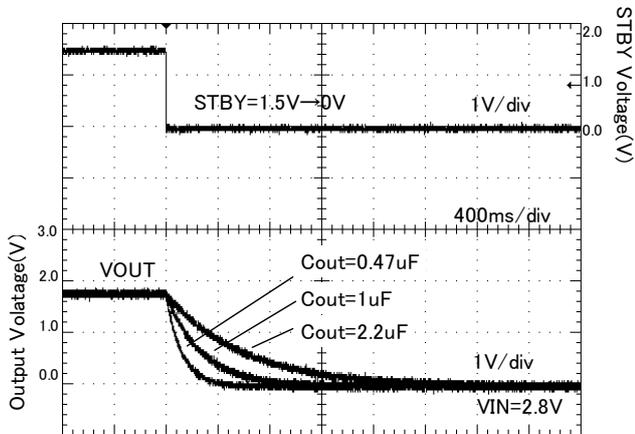
Figure 20. Discharge time ( Rout = none )
