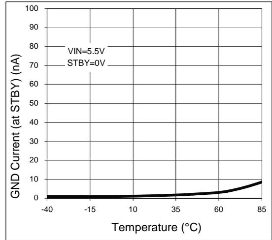
Figure 35. GND Current (at STBY) vs. Temperature
