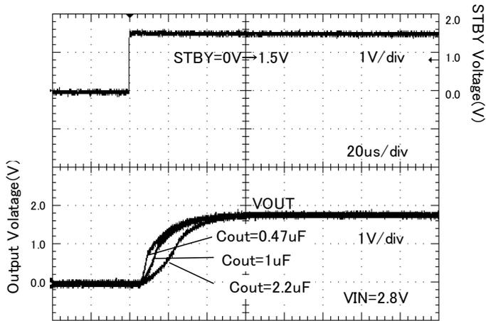
Figure 18. Startup time ( Rout = none )
