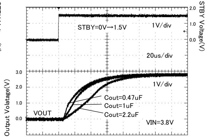
Figure 43. Startup time ( Rout = 14 ohm )
