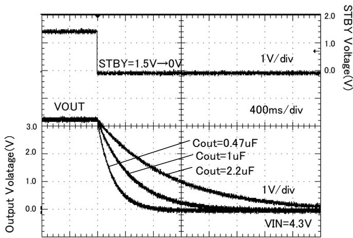
Figure 92. Discharge time ( Rout = none )
