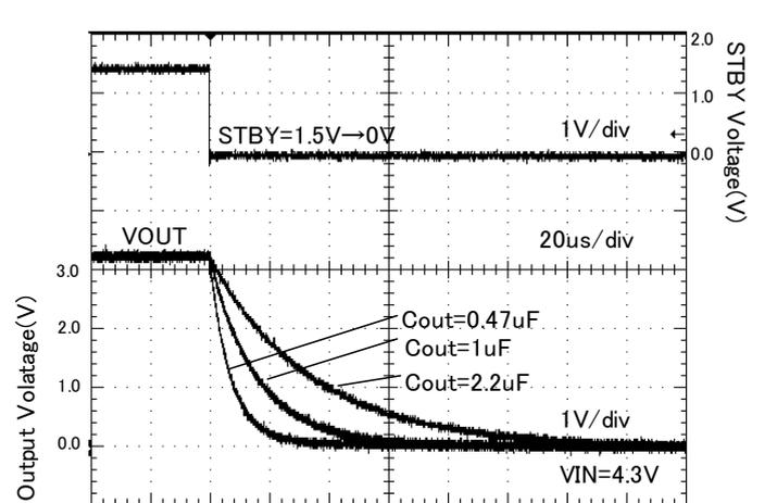
Figure 93. Discharge time ( Rout = 16.5 ohm )
