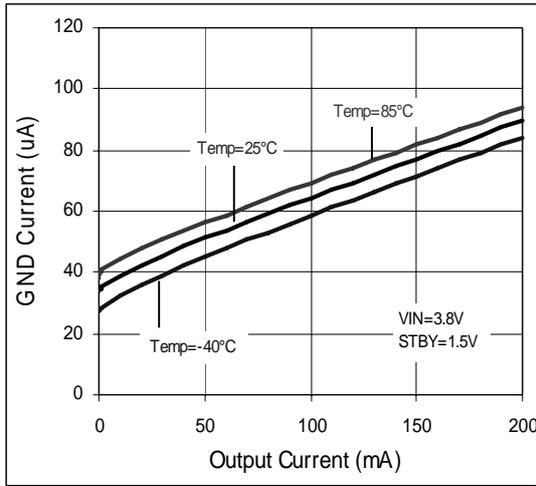
Figure 30. GND Current vs. Output Current
