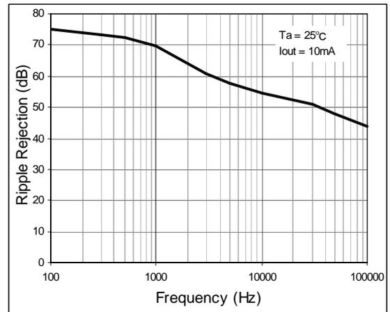
Figure 63. Ripple Rejection vs. Frequency
