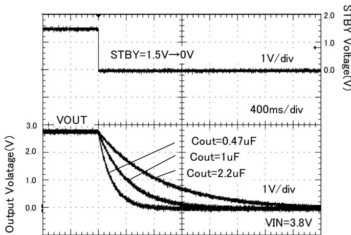
Figure 44. Discharge time ( Rout = none )
