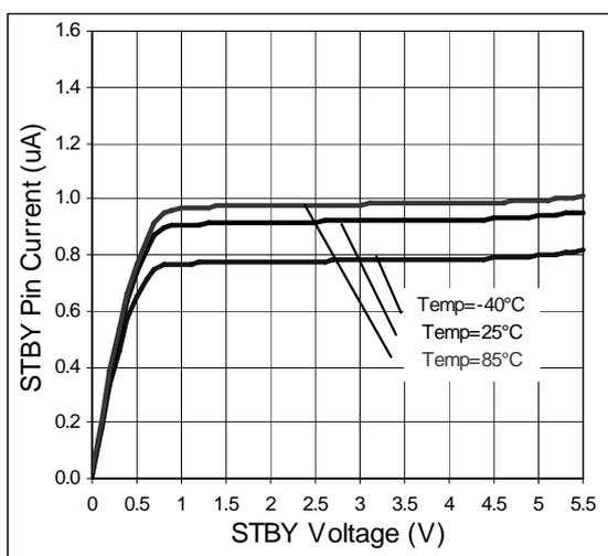
Figure 13. STBY Pin Current vs. STBY Pin Voltage
