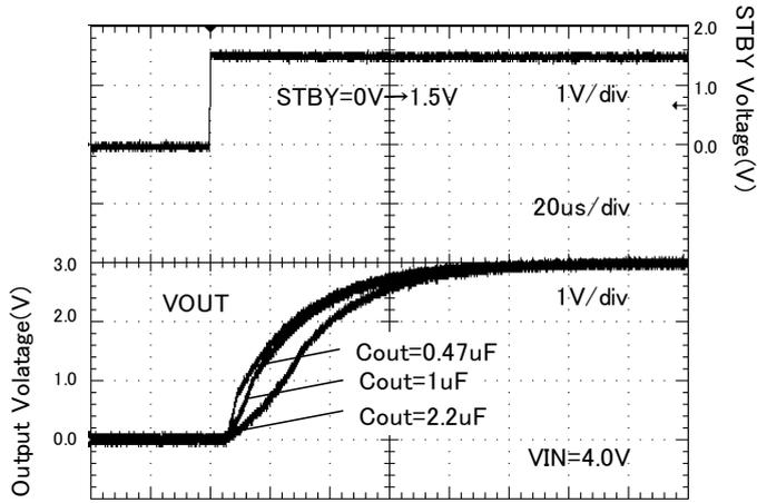
Figure 66. Startup time ( Rout = none )
