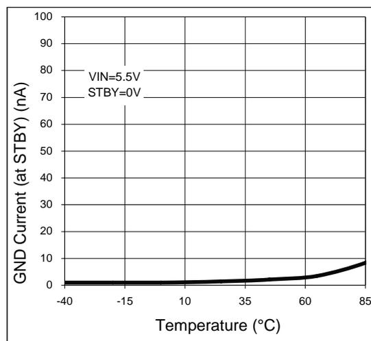
Figure 12. GND Current (at STBY) vs. Temperature
