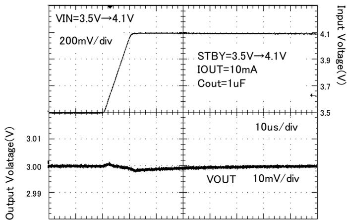
Figure 72. Line response ( $V_{in} = 3.5\text{V} \rightarrow 4.1\text{V}$ )
