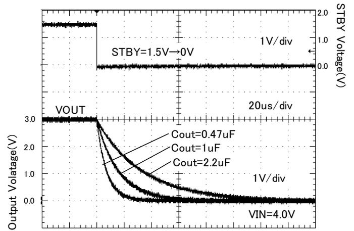
Figure 69. Discharge time ( Rout = 15 ohm )
