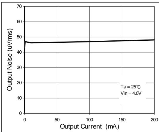
Figure 64. Output Noise vs. Output Current
