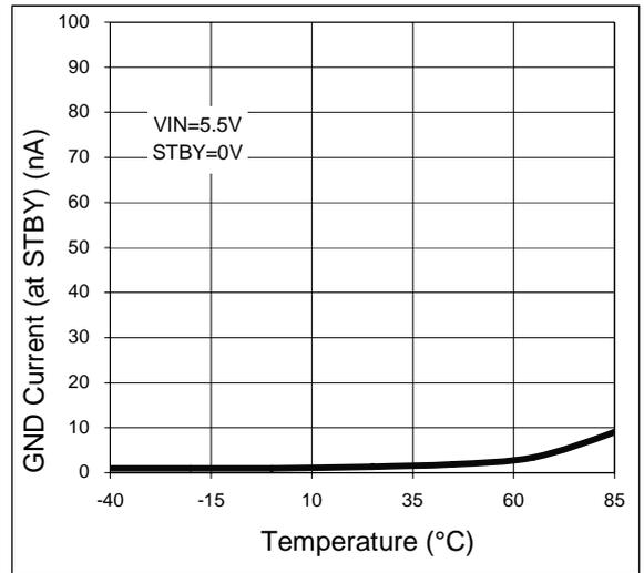
Figure 83. GND Current (at STBY) vs. Temperature
