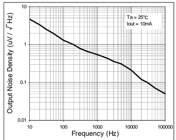
Figure 65. Output Noise Density vs. Frequency
