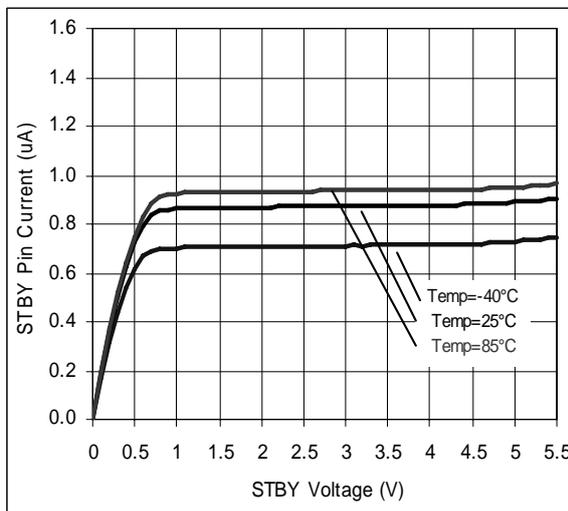
Figure 36. STBY Pin Current vs. STBY Voltage
