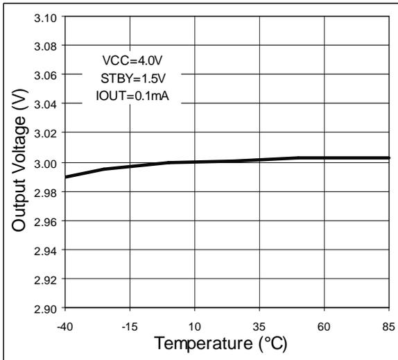
Figure 56. Output Voltage vs. Temperature
