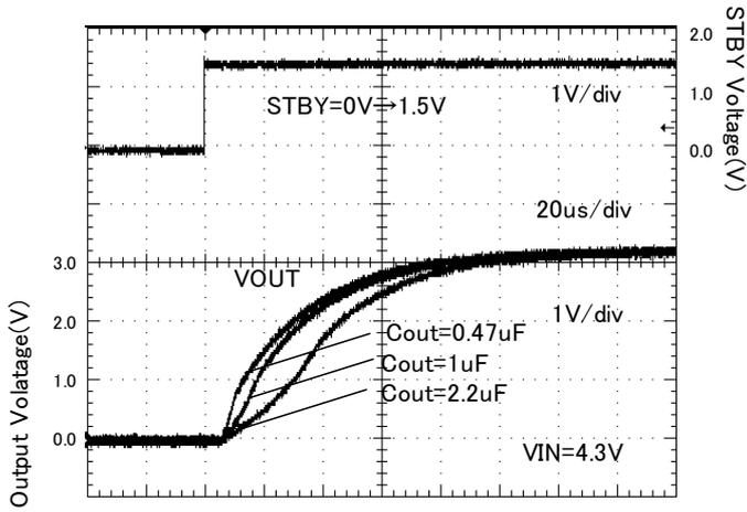
Figure 90. Startup time ( Rout = none )
