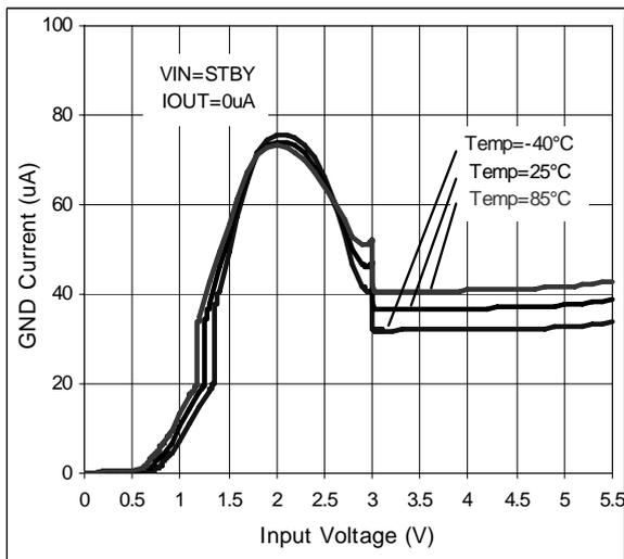
Figure 52. GND Current vs. Input Voltage
