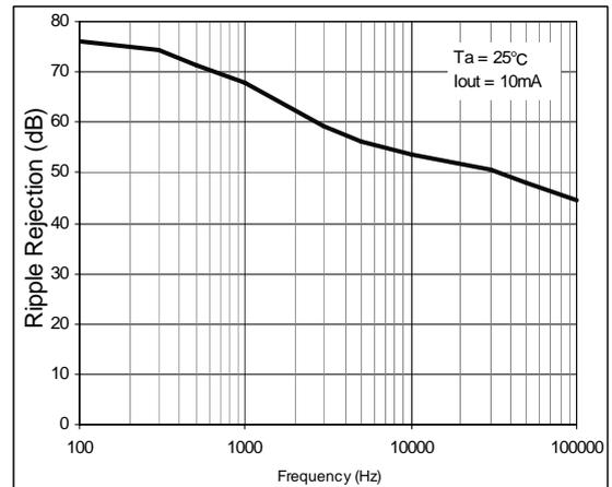
Figure 87. Ripple Rejection vs. Frequency
