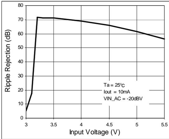
Figure 62. Ripple Rejection vs. Input Voltage
