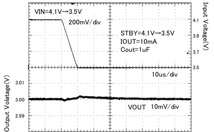
Figure 73. Line response ( $V_{in} = 4.1\text{V} \rightarrow 3.5\text{V}$ )
