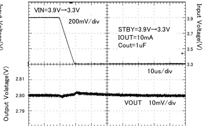
Figure 49. Line response ( $V_{in} = 3.9\text{V} \rightarrow 3.3\text{V}$ )
