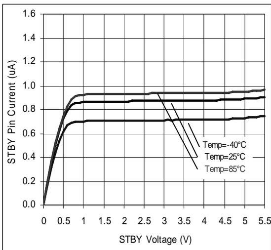
Figure 60. STBY Pin Voltage vs. STBY Pin Current
