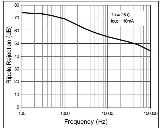
Figure 39. Ripple Rejection vs. Frequency
