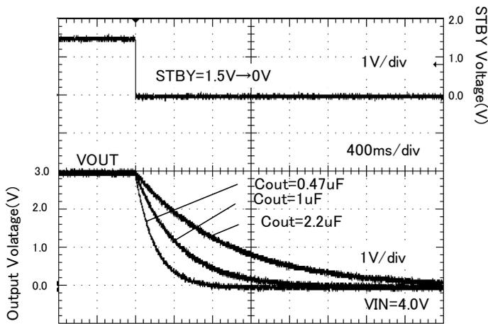
Figure 68. Discharge time ( Rout = none )
