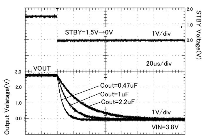
Figure 45. Discharge time ( Rout = 14 ohm )
