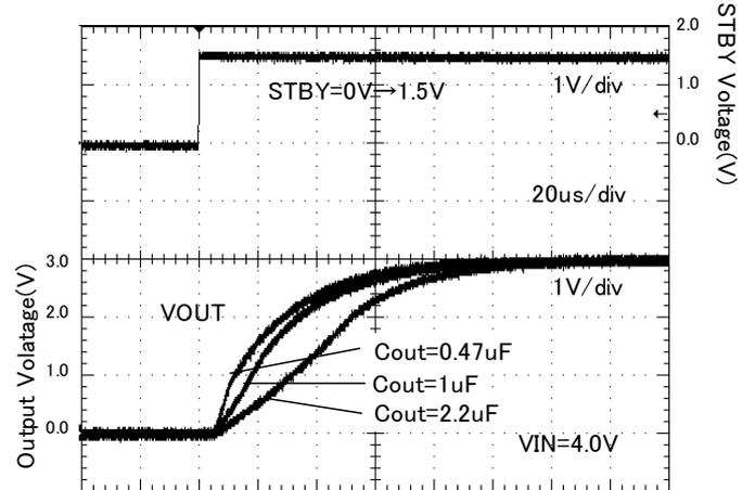
Figure 67. Startup time ( Rout = 15 ohm )
