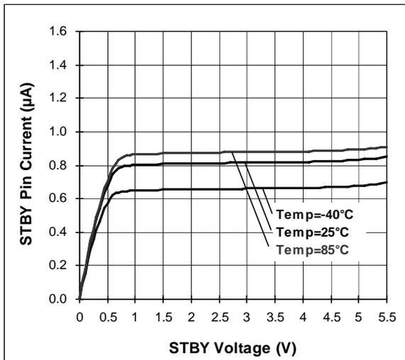
Figure 84. STBY Pin Current vs. STBY Voltage
