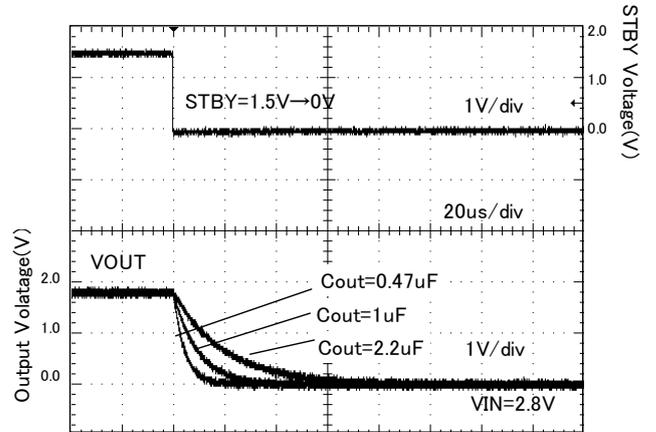
Figure 21. Discharge time ( Rout = 9 ohm )
