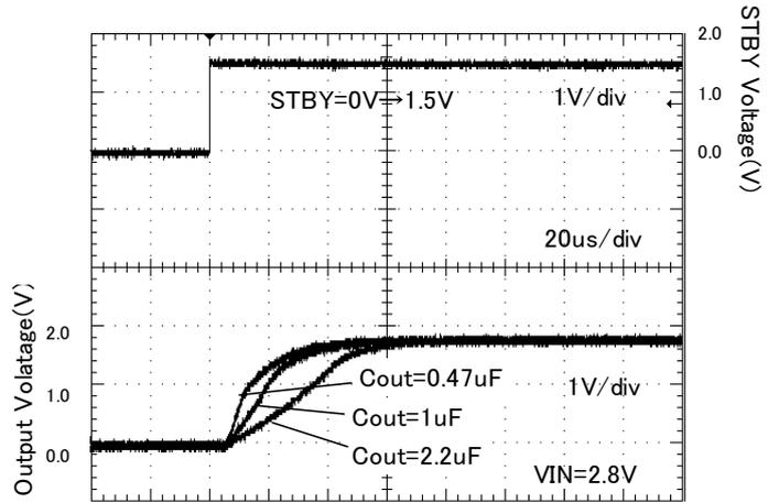
Figure 19. Startup time ( Rout = 9 ohm )
