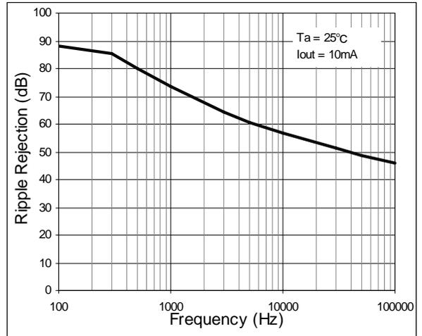
Figure 15. Ripple Rejection vs. Frequency
