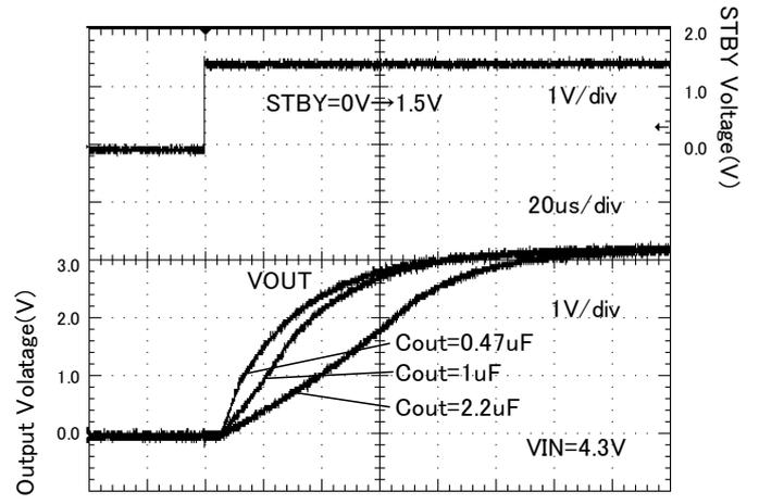
Figure 91. Startup time ( Rout = 16.5 ohm )
