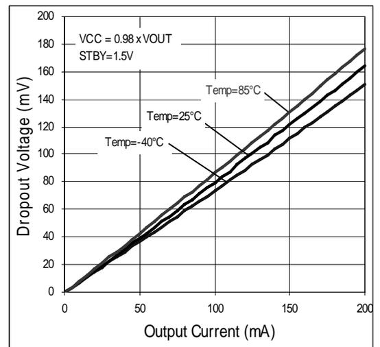
Figure 61. Dropout Voltage vs. Output Current
