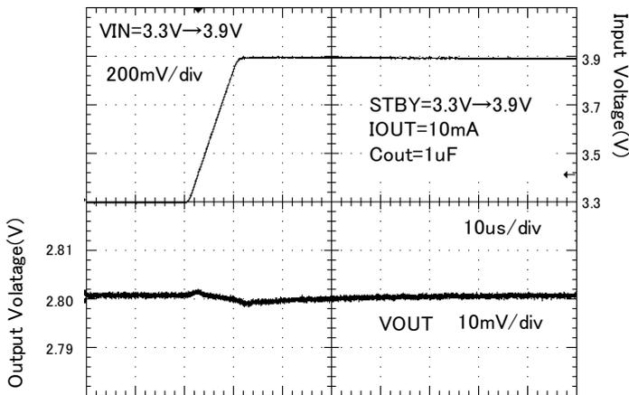
Figure 48. Line response ( $V_{in} = 3.3\text{V} \rightarrow 3.9\text{V}$ )
