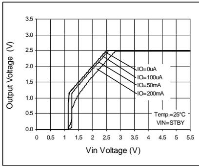
Fig. 63 Output Voltage
