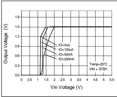
Fig. 5 Output Voltage
