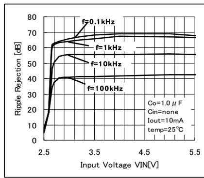
Fig. 76 Ripple Rejection VS VIN
