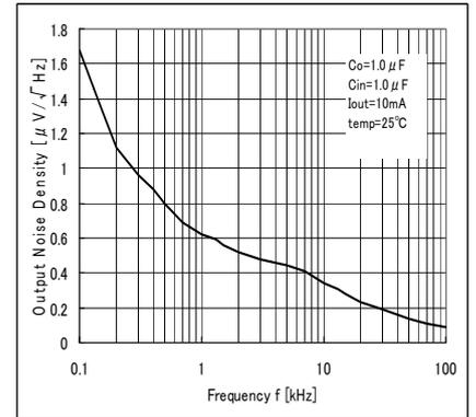
Fig. 164 Output Noise Spectral Density VS Freq.
