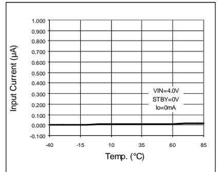
Fig. 132 IIGND vs Temp (STBY)
