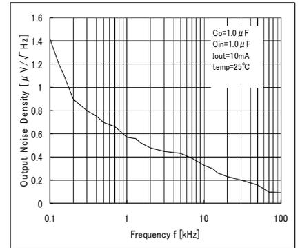
Fig. 135 Output Noise Spectral Density VS Freq.
