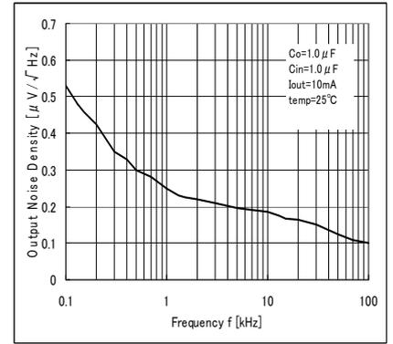
Fig. 19 Output Noise Spectral Density vs Freq.
