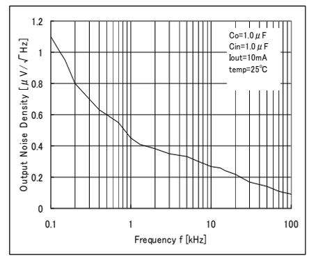
Fig. 77 Output Noise Spectral Density VS Freq.
