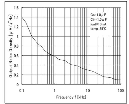
Fig. 106 Output Noise Spectral Density VS Freq.
