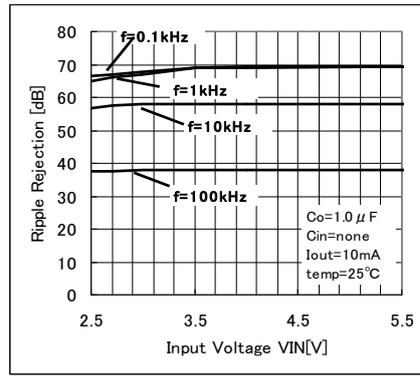
Fig. 18 Ripple Rejection vs VIN (Iout=10mA)
