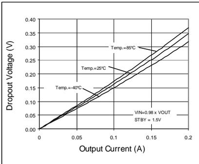
Fig. 95 Dropout Voltage
