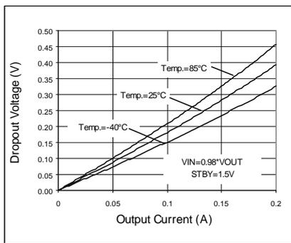
Fig. 66 Dropout Voltage
