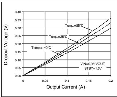
Fig. 124 Dropout Voltage
