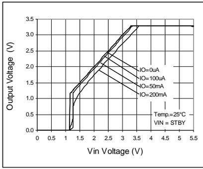
Fig. 150 Output Voltage
