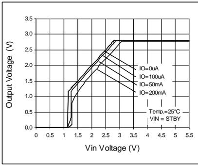
Fig. 92 Output Voltage
