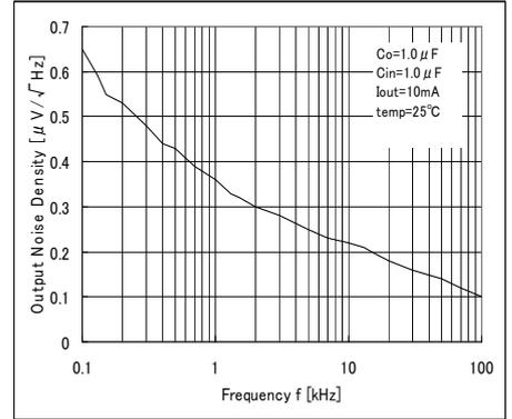
Fig. 48 Output Noise Spectral Density VS Freq.
