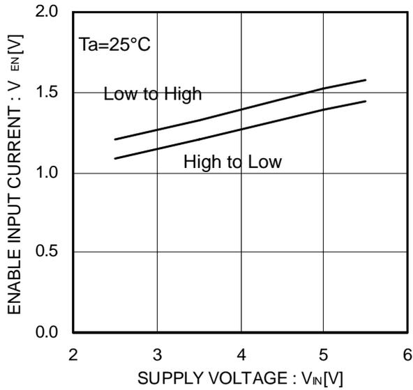
Figure 8. EN/ $\overline{EN}$  入力電圧
