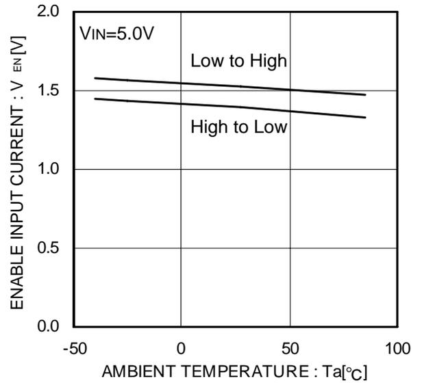
Figure 9. EN/ $\overline{EN}$  入力電圧
