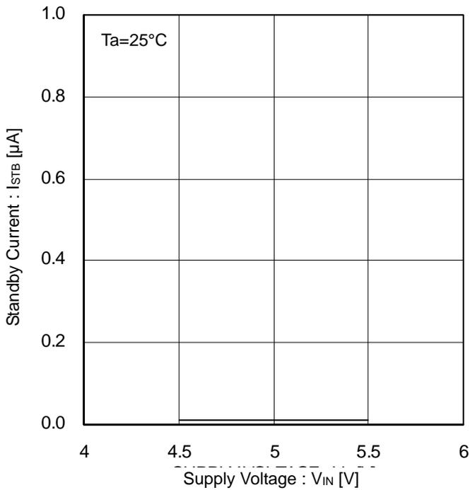
Figure 8. Standby Current vs Supply Voltage
