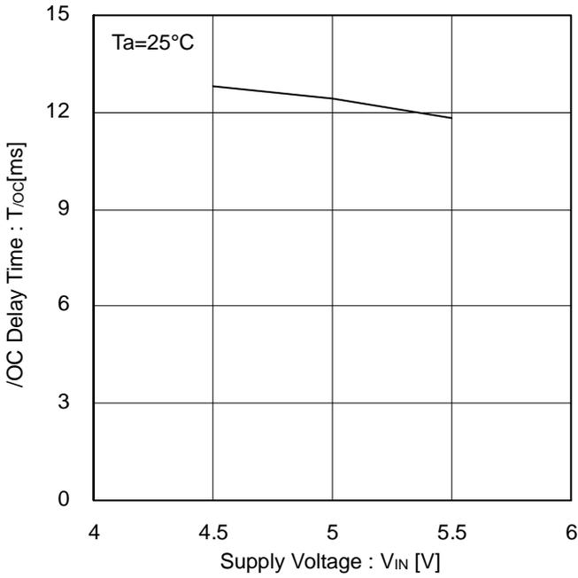
Figure 30. /OC Delay Time vs Supply Voltage
