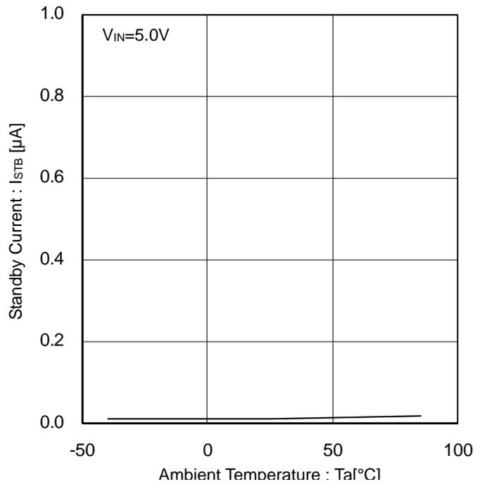
Figure 9. Standby Current vs Ambient Temperature
