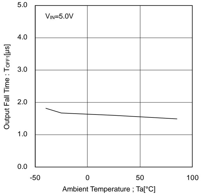
Figure 27. Output Fall Time vs Ambient Temperature
