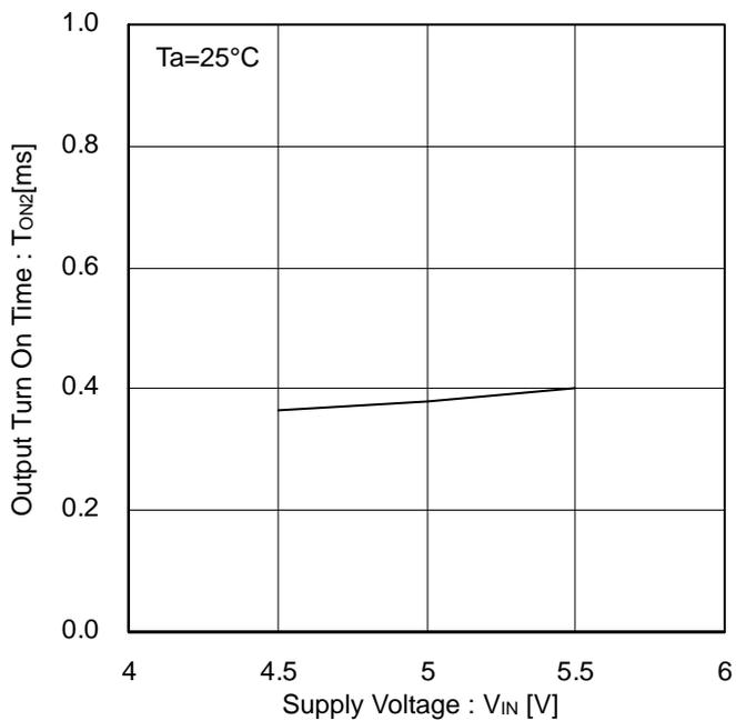
Figure 24. Output Turn-on Time vs Supply Voltage
