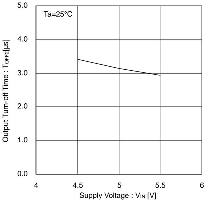
Figure 28. Output Turn-off Time vs Supply Voltage
