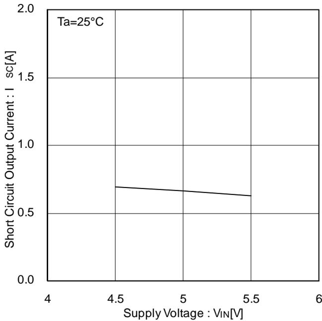
Figure 16. Short Circuit Output Current vs Supply Voltage
