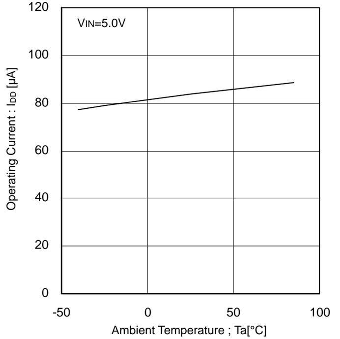
Figure 7. Operating Current vs Ambient Temperature
