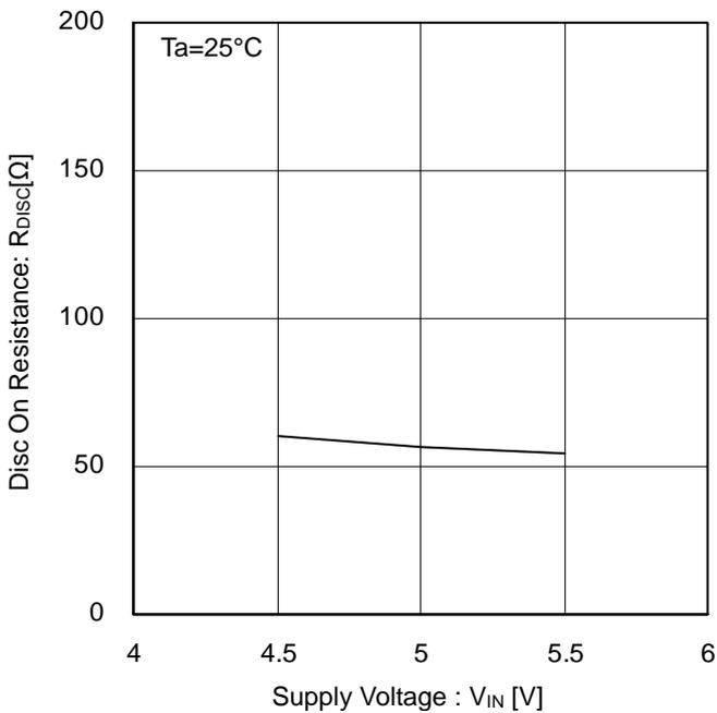
Figure 32. Discharge On Resistance vs Supply Voltage
