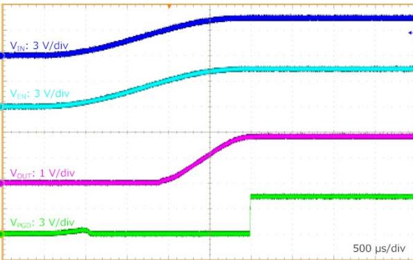
Figure 62.  $R_{Load} = 0.9\ \Omega$  VIN 起動波形
