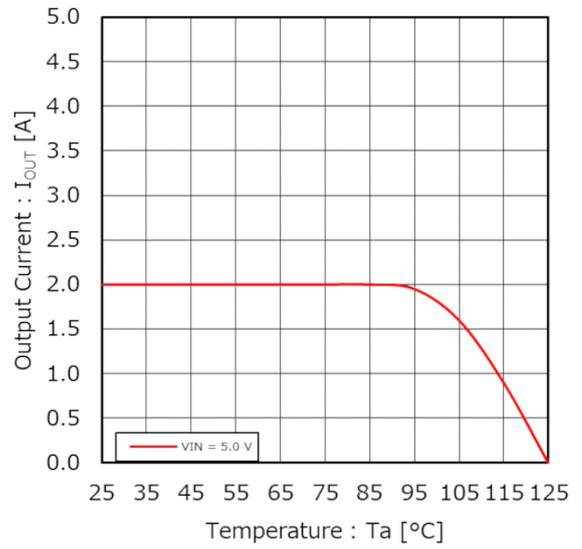
Figure 69. Thermal Derating (V<sub>OUT</sub> = 3.3 V)
