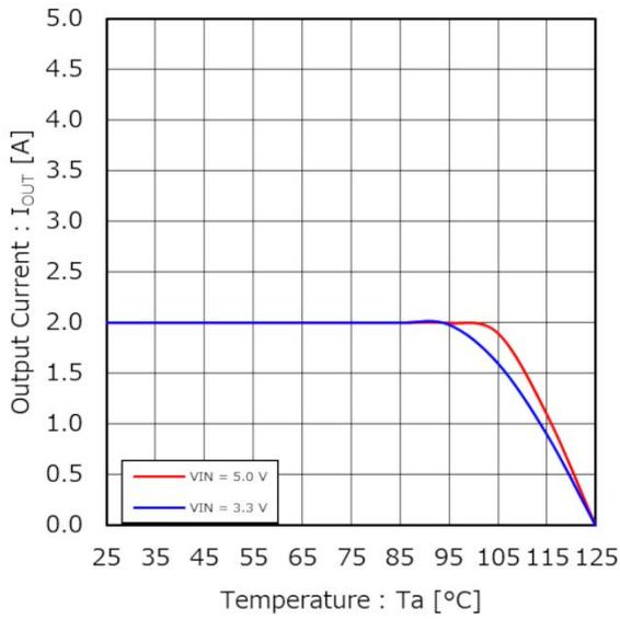
Figure 68. Thermal Derating (V<sub>OUT</sub> = 1.8 V)
