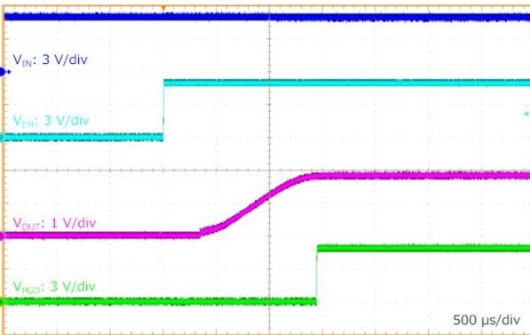
Figure 58.  $R_{Load} = 0.9\ \Omega$  EN 起動波形
