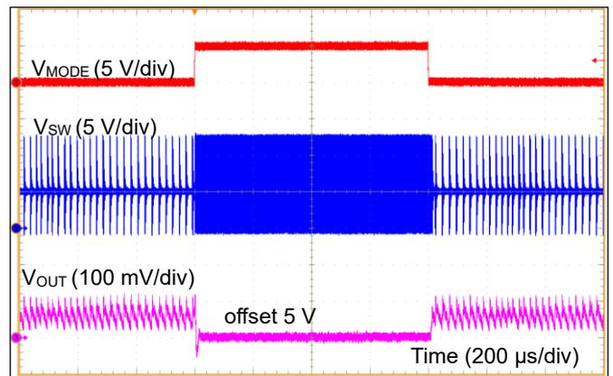
Figure 44. MODE ON/OFF 応答
