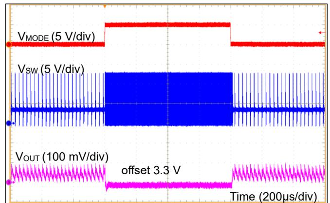
Figure 61. MODE ON/OFF 応答
