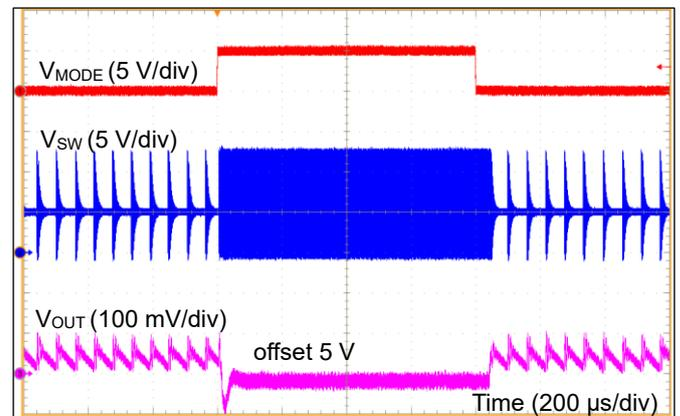
Figure 78. MODE ON/OFF 応答
