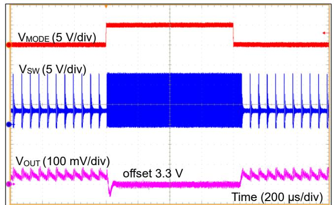
Figure 91. MODE ON/OFF 応答
