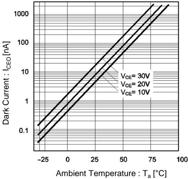
Fig.10 Output Characteristics
