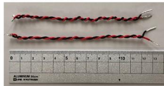
(c) Twisted cable with 100 ohm damping
