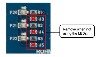
Fig. 4 Jumper-chip removal of LEDs
