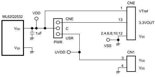
Fig. 2 Power Circuit
