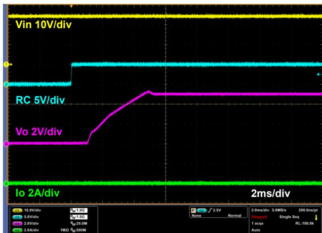
Figure 11-24. Startup Waveform
