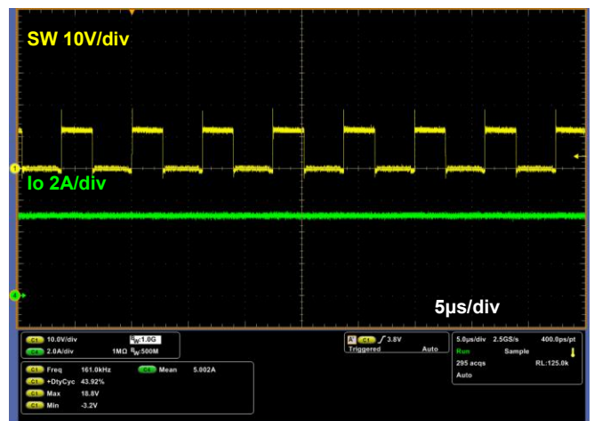
Figure 11-11. Switching Waveform ( V_{in}=12V , V_o=5V , I_o=5A )
