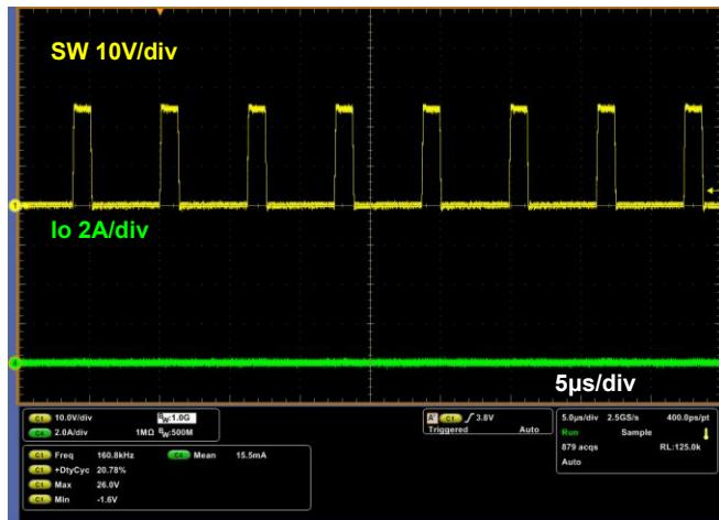
Figure 11-12. Switching Waveform
