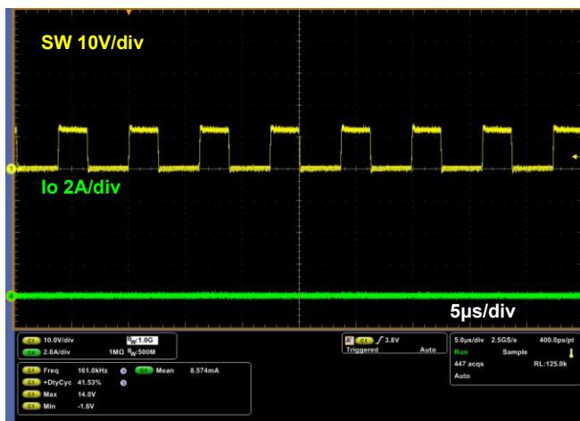
Figure 11-10. Switching Waveform
