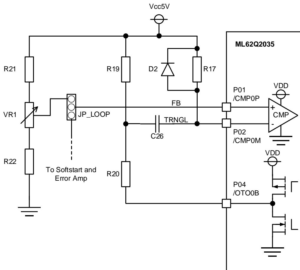
Figure 4-4. Triangle waveform generator and surrounding circuit
