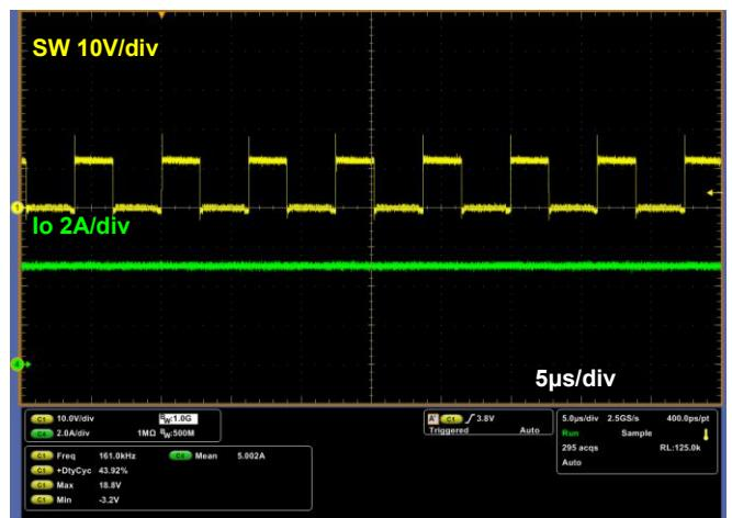
Figure 11-11. Switching Waveform
