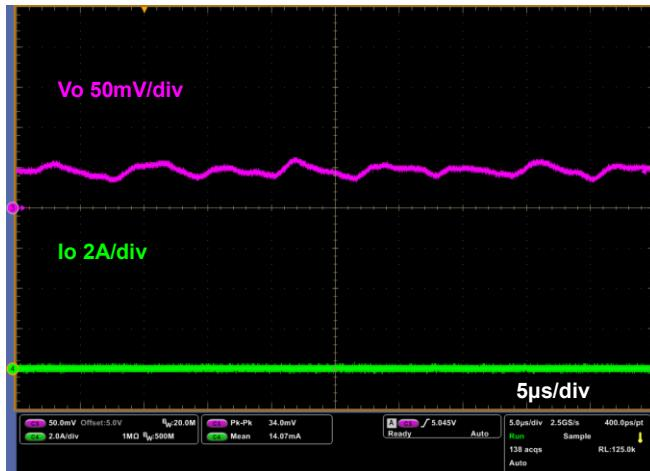
Figure 11-8. Output Ripple Voltage
