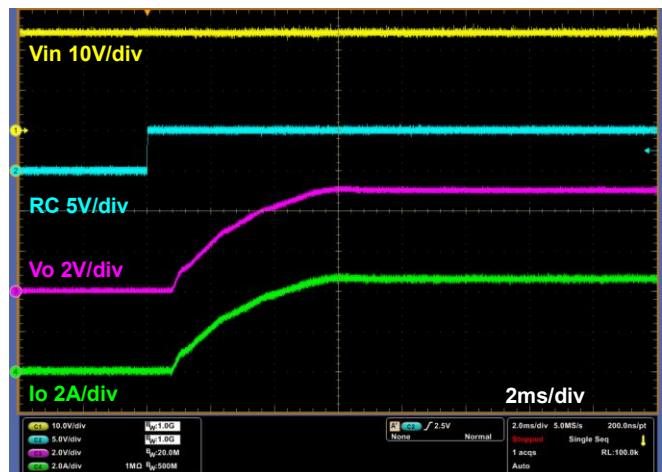
Figure 11-25. Startup Waveform
