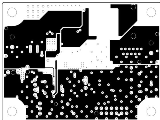
Figure 9-5. Middle2 Layer Layout (Top View)
