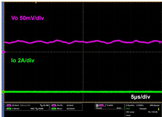
Figure 11-6. Output Ripple Voltage
