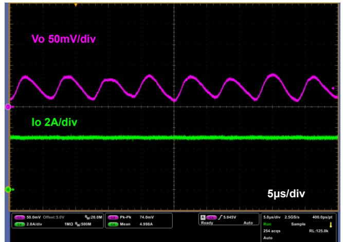
Figure 11-9. Output Ripple Voltage
