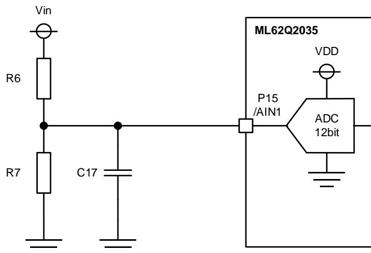
Figure 4-6. Input voltage detection block
