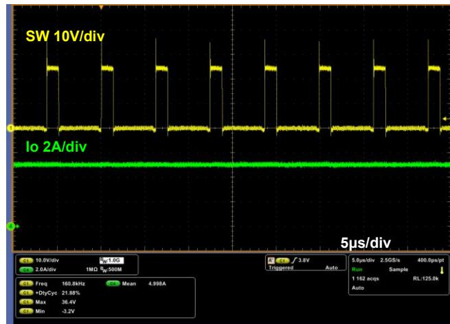
Figure 11-13. Switching Waveform
