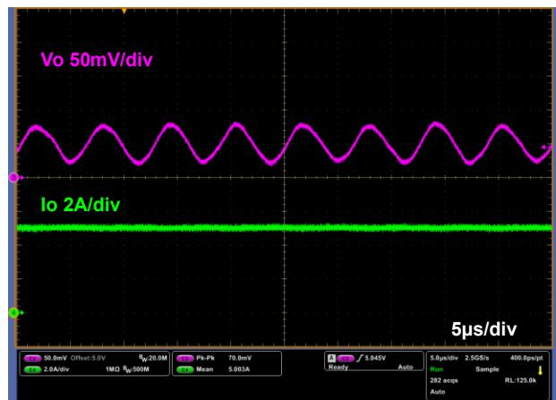
Figure 11-7. Output Ripple Voltage
