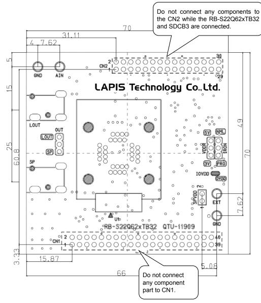
Figure 7 PCB layout
