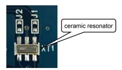
Figure 4 Ceramic resonator
