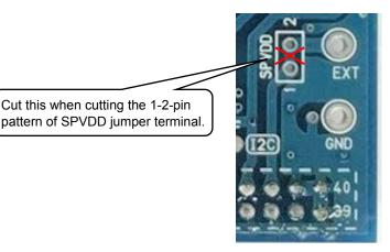
Figure 3 SPVDD jumper terminal
