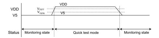
● Definition of overvoltage detection/release threshold voltage range and step The overvoltage detection/release thresholds can be defined as shown in the following table. Since some combinations are unavailable, contact us for detail.
