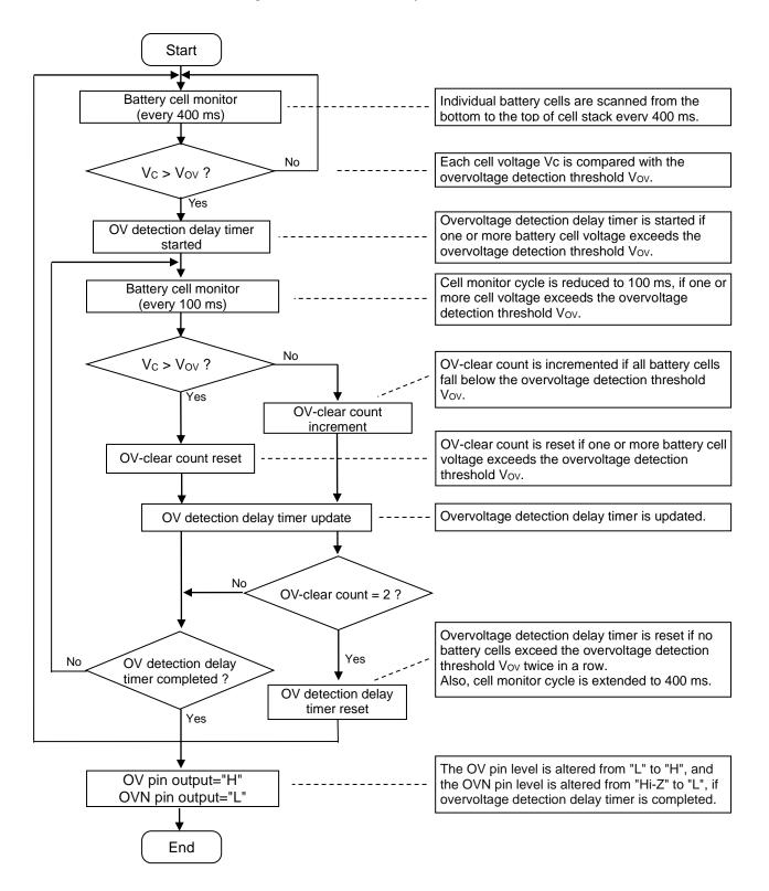
• Overvoltage Release Flow Below is the operation flow chart at overvoltage release. Overvoltage state is assumed initially.
