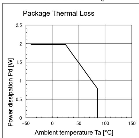
Package thermal loss tolerance decreases with increased ambient temperature Ta as in the left diagram. Make sure that the thermal loss tolerance is not exceeded especially when the output current on the VREG pin is high.
