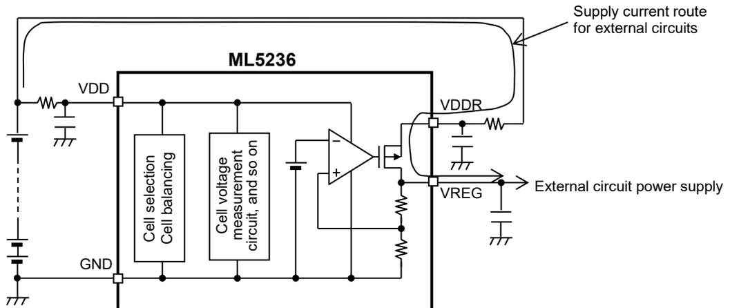
The maximum output current of the built-in regulator (VREG output) is 10mA. If the consumption current of the external circuits exceeds 10mA, configure an external current boost circuit with Pch-FET as in the diagram below.
