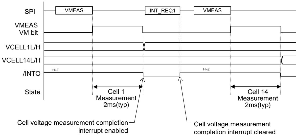
Scan measurement timing diagram (Cell 13 to Cell 14 scanned)
