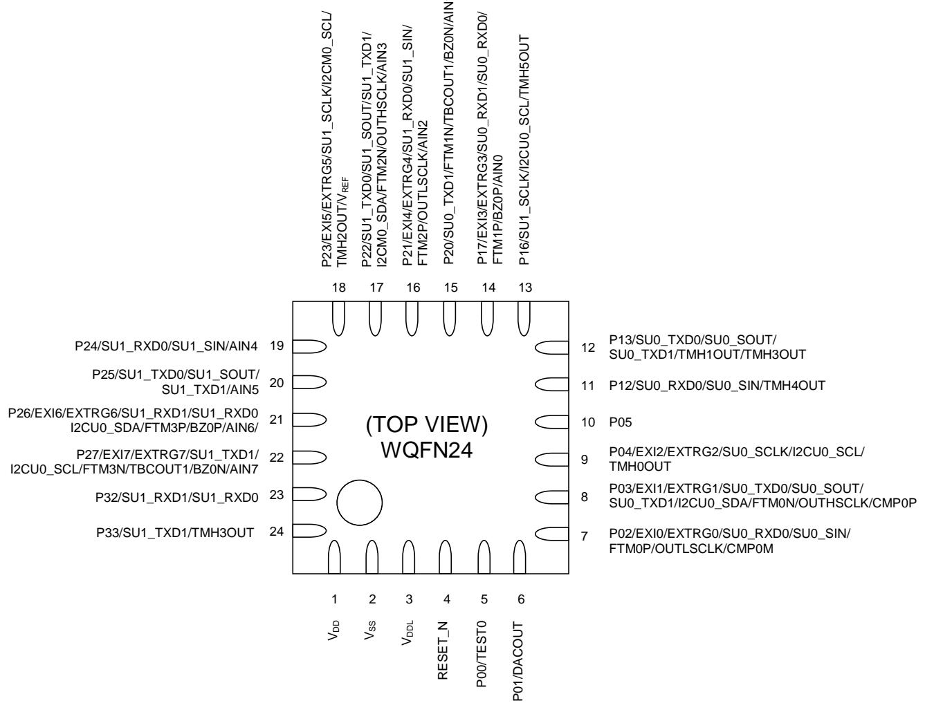
Figure 6 Pin Layout of ML62Q1245E/1246E/1247E 24pin WQFN Package
