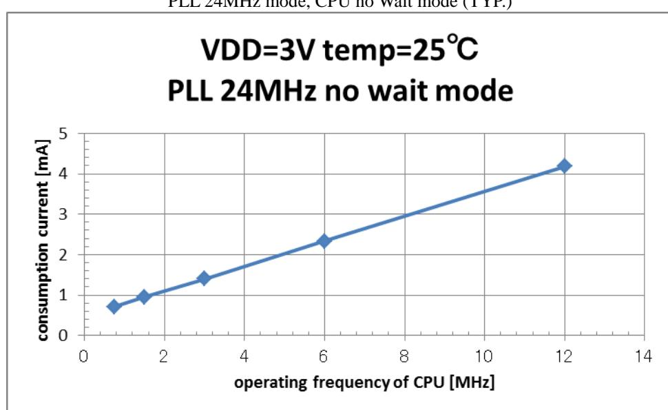
VDD=3V, temp=25°C, stop the clock supply to peripherals.
