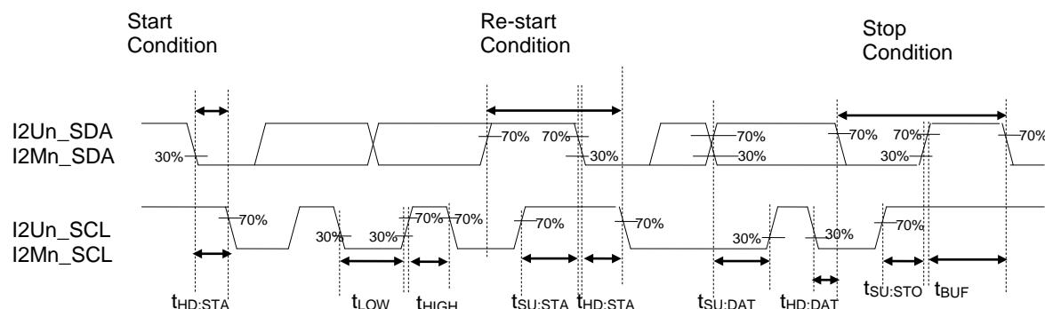
**Fast Mode 400kHz**(V<sub>DD</sub>=1.8 to 5.5V, V<sub>SS</sub>=0V, Ta=-40 to +105°C, unless otherwise specified)
