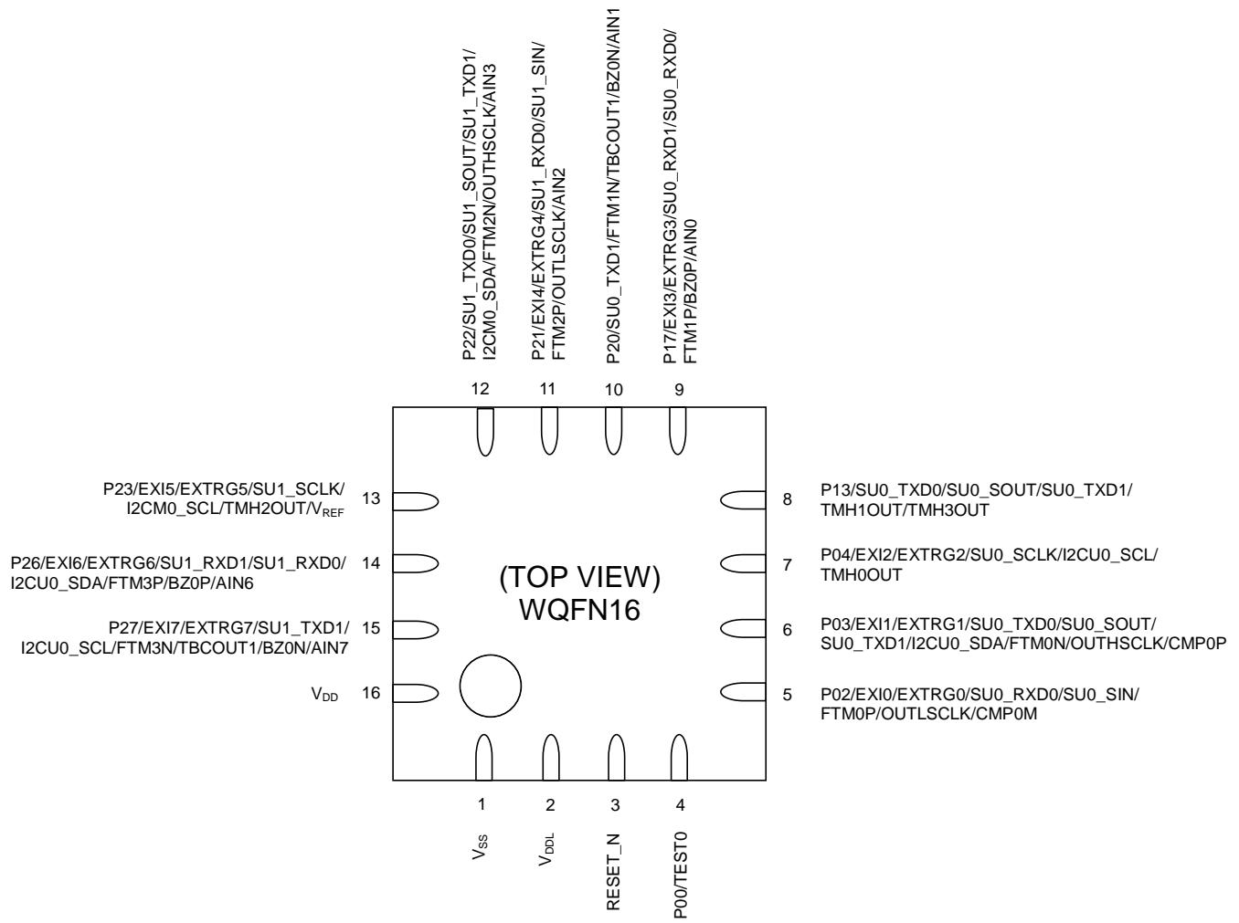
Figure 4 Pin Layout of ML62Q1223E/1224E/1225E 16pin WQFN Package
