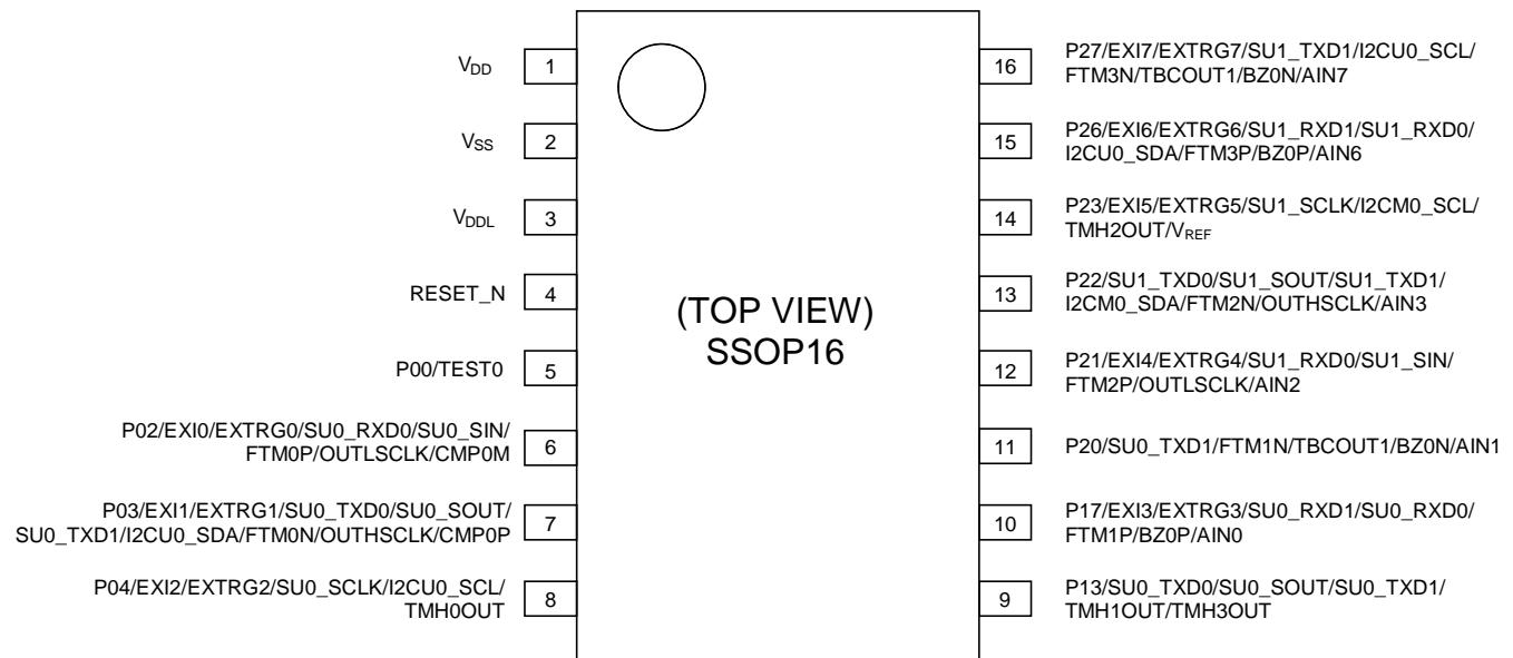
Figure 3 Pin Layout of ML62Q1223E/1224E/1225E 16pin SSOP Package
