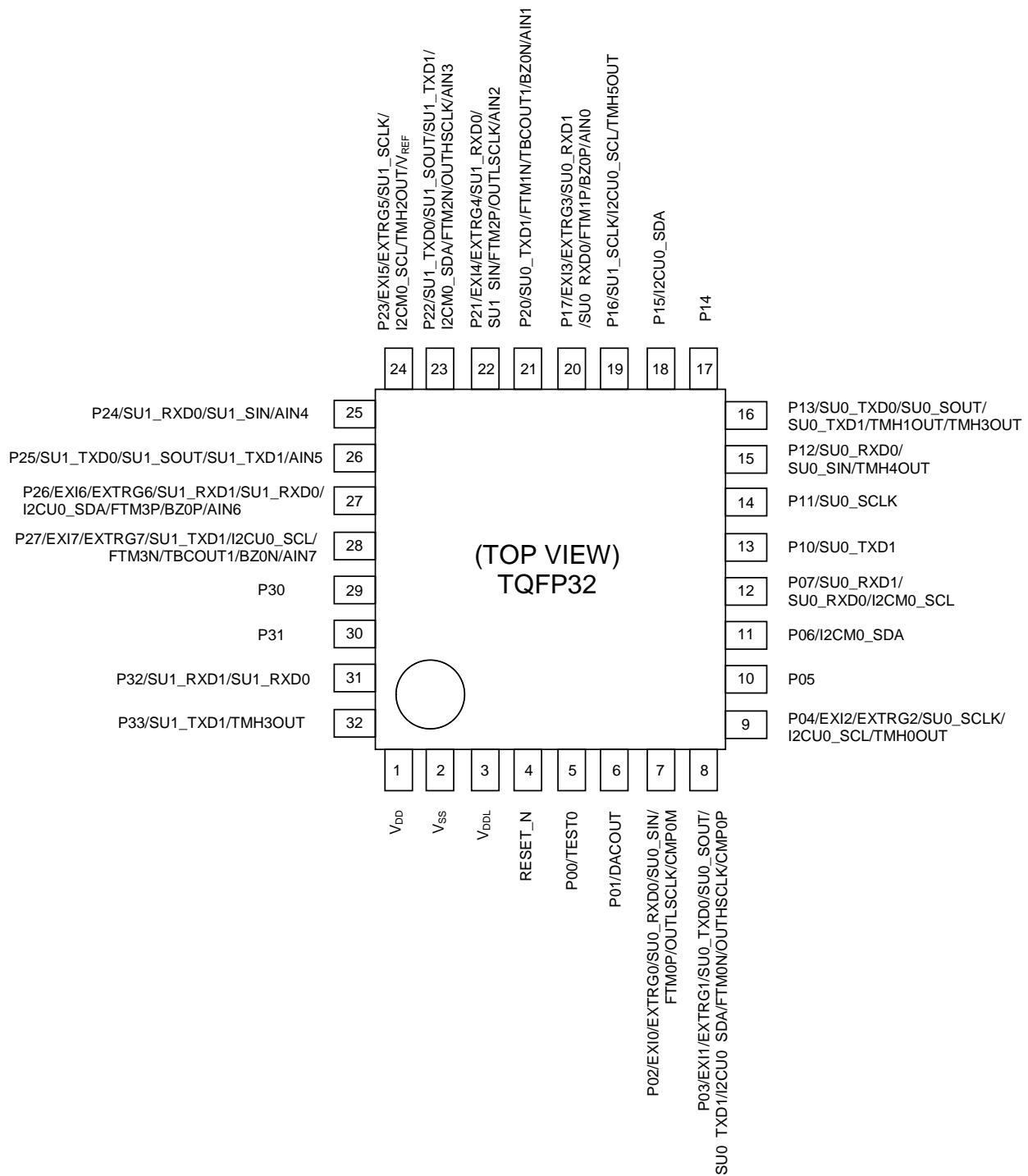
Figure 7 Pin Layout of ML62Q1265E/1266E/1267E 32pin TQFP Package
