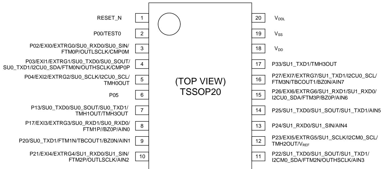
Figure 5 Pin Layout of ML62Q1233E/1234E/1235E 20pin TSSOP Package
