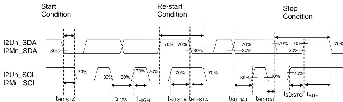
**1Mbps Mode**(V<sub>DD</sub>=2.7 to 5.5V, V<sub>SS</sub>=0V, Ta=-40 to +105°C, unless otherwise specified)
