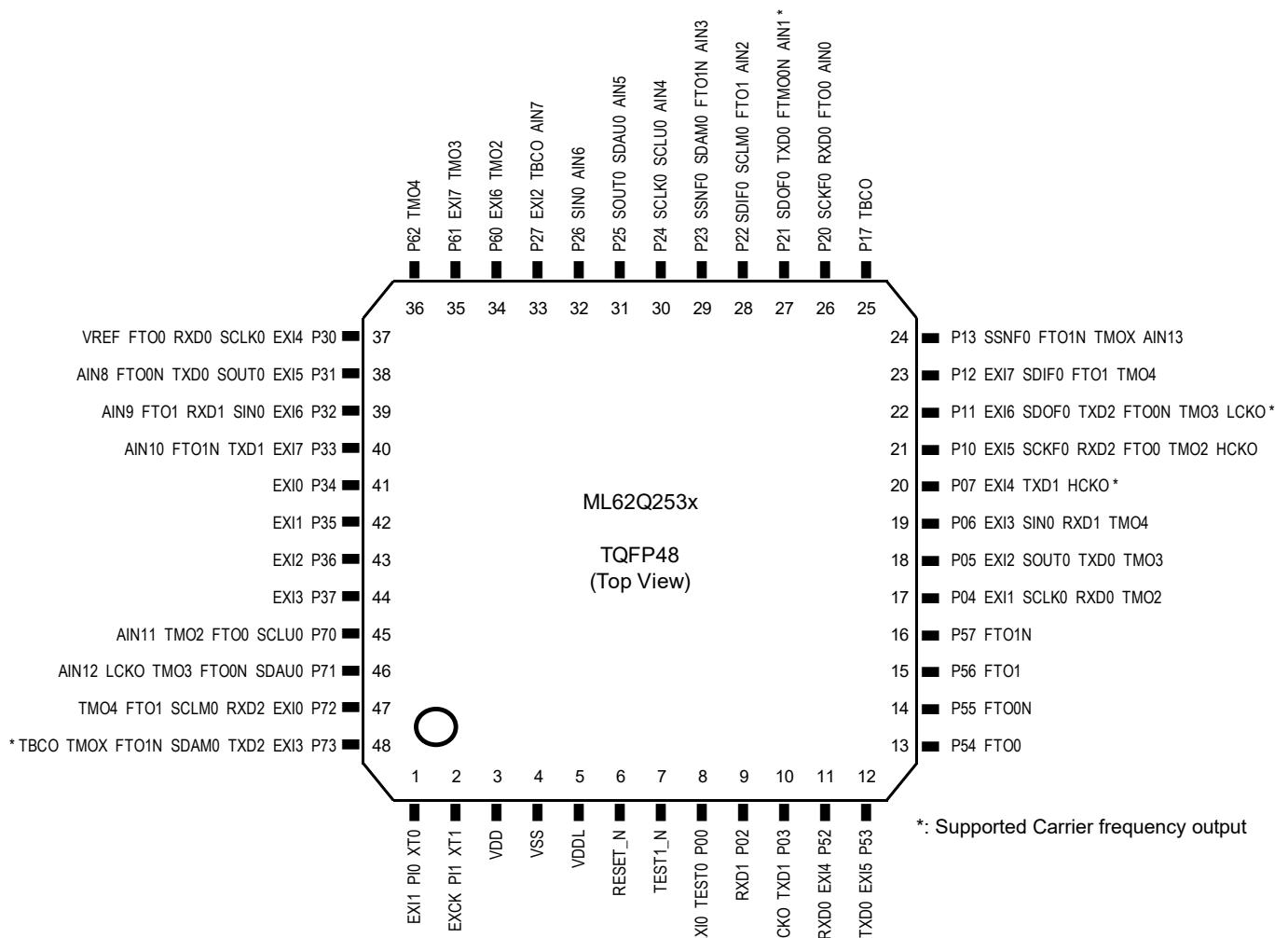
Fig.3-1 48 pin TQFP
