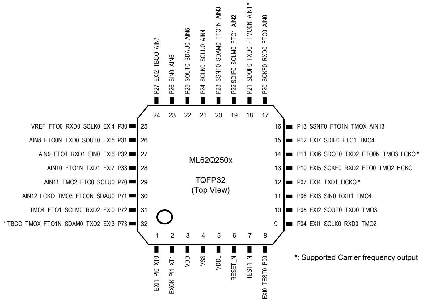
Fig.3-4 32 pin TQFP
