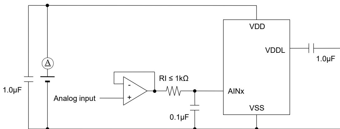
The current flows during the SA-ADC sampling as it takes charging. Make the output impedance of the analog signal source 1kΩ or smaller. Also, putting 0.1µF capacitor on the ADC input pin is recommended for noise reduction.
